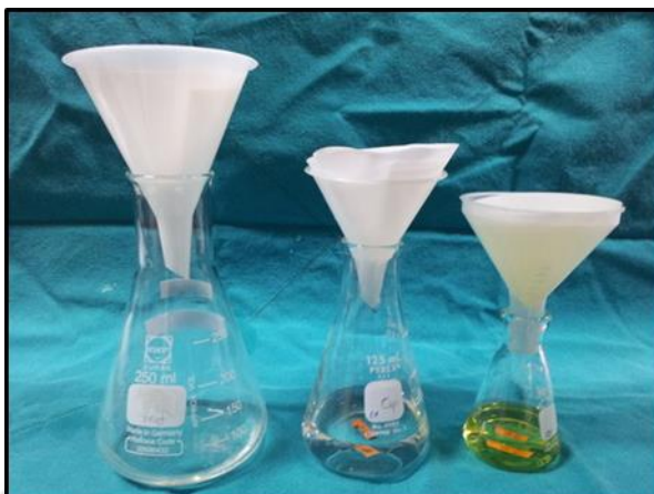
Figure 16 Preparation of stock solution of 3Mix. The solution of each antibiotic was filtered using 2.00 micron pore-size filter paper.
