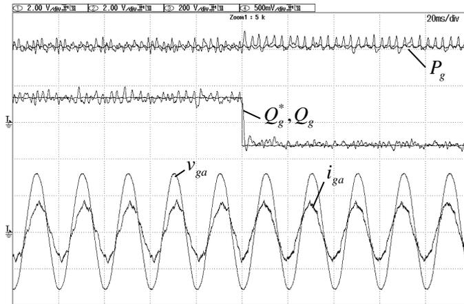
Figure 3.22 Experiment waveforms of dynamic response operation in the rectifying mode.
