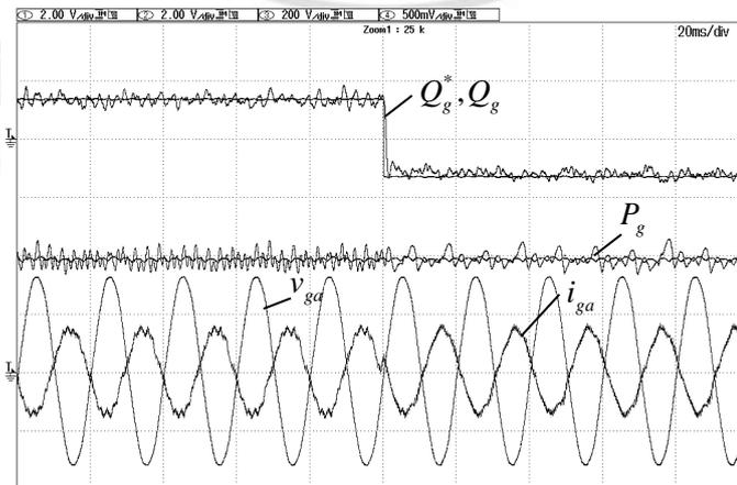
Figure 3.21 Experiment waveforms of dynamic response operation in the inverting mode.
