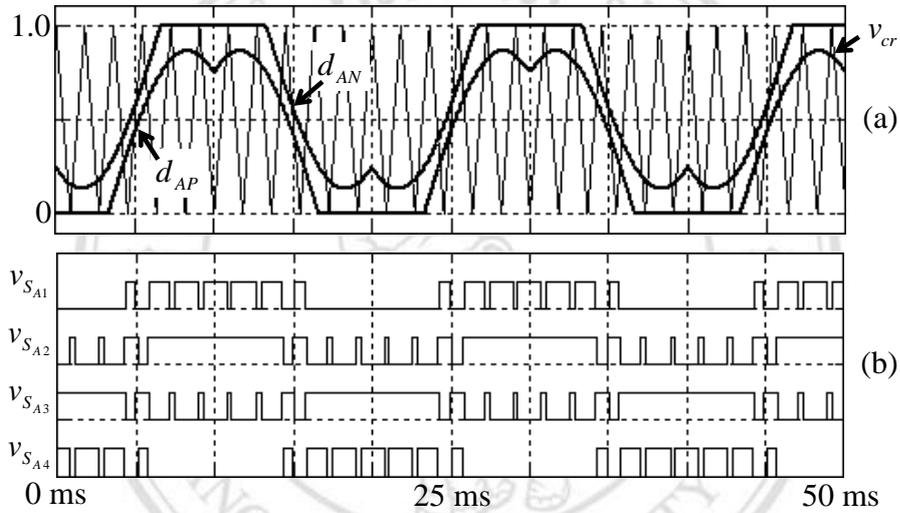
Figure 3.7 Simulation waveforms for leg A (a) the modified duty cycles  $d_{AP}$  and  $d_{AN}$
