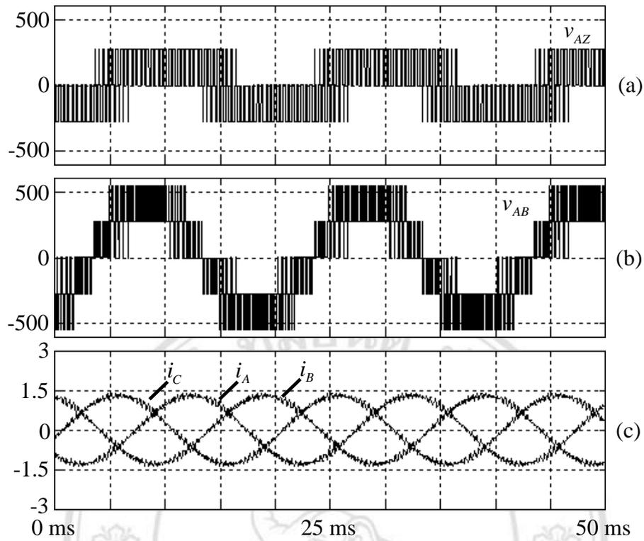
Figure 3.9 Simulation waveforms at high modulation index,  $m_a = 0.8$  (a) pole voltage
