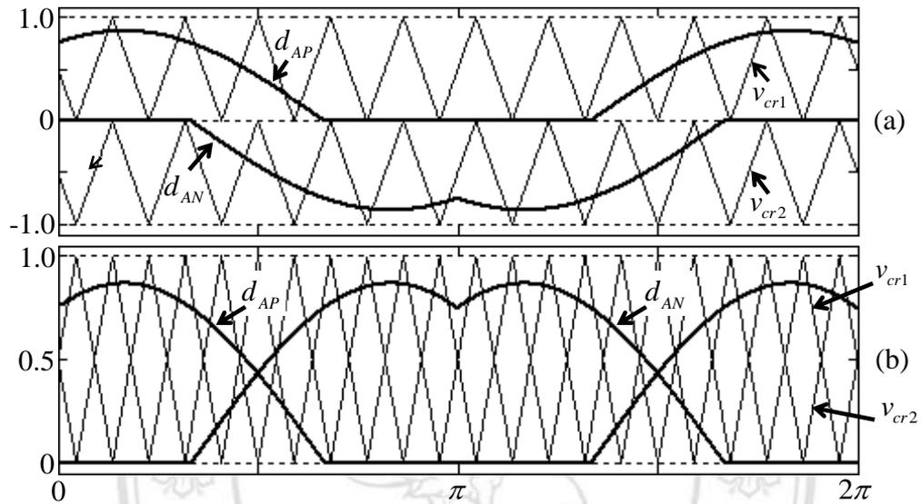
Figure 3.6 The modified duty cycles for leg A of the conventional CB-PWM strategies
