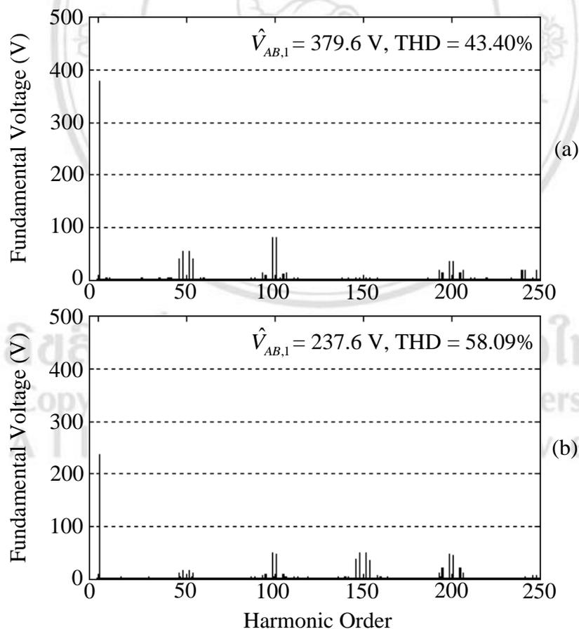
Figure 3.11 Simulation harmonic spectrum of line-to-line voltage  $v_{AB}$  with proposed CB-PWM strategy (a)  $m_a = 0.8$  (b)  $m_a = 0.5$ .
