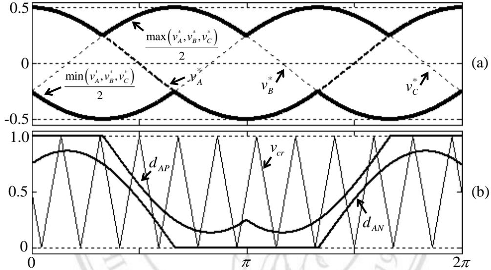
Figure 3.5 The modified duty cycles for leg  $A$  of the proposed CB-PWM strategy under the condition of  $m_a = 1.0$ ,  $\text{sgn} = +1$ , and  $\delta = +1$ .
