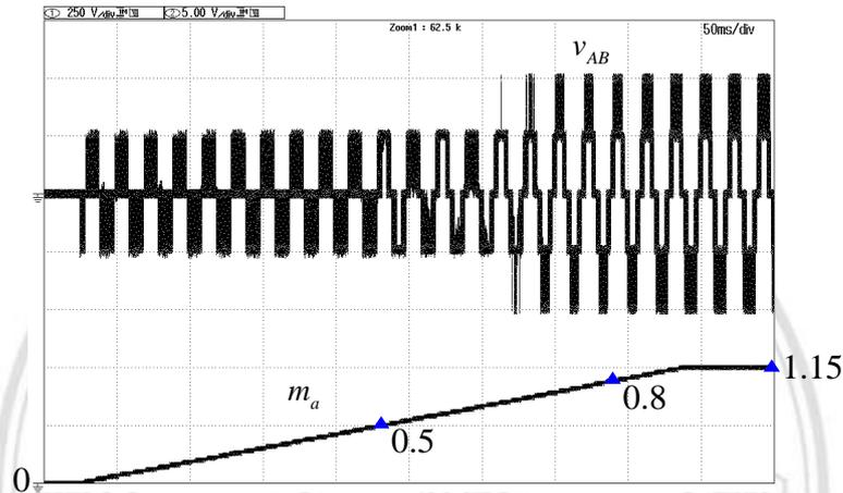
Figure 3.14 Experimental waveforms of dynamic response operation for a ramp modulation index reference: the line-to-line voltage  $v_{AB}$  (Scale: 250 V/div) and the modulation index  $m_a$  (Scale: 5 V/div).
