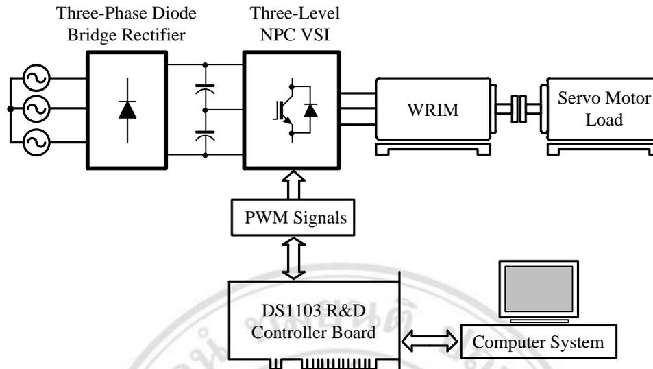
Figure 3.12 Experimental set-up.
