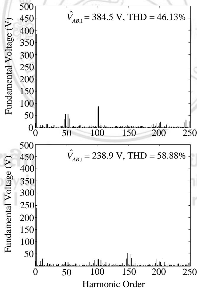
Figure 3.17 Experimental harmonic spectrum of line-to-line voltage with the proposed CB-PWM strategy (a)  $m_a = 0.8$  (b)  $m_a = 0.5$ .
