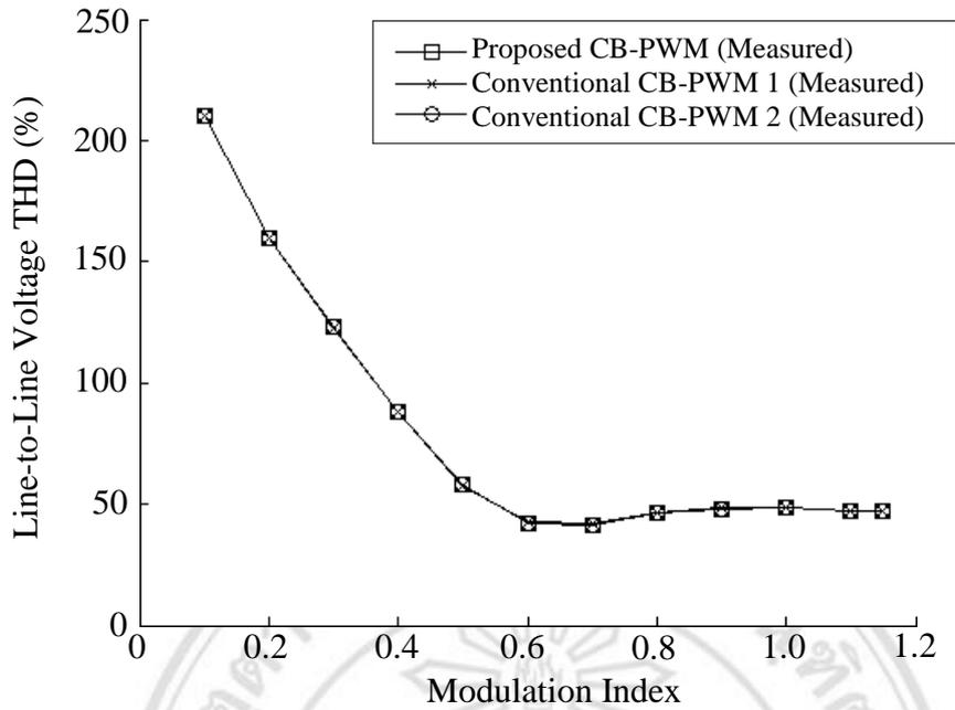
Figure 3.18 THD of the output line-to-line voltages with modulation index of the three-level NPC VSI for different CB-PWM strategies.
