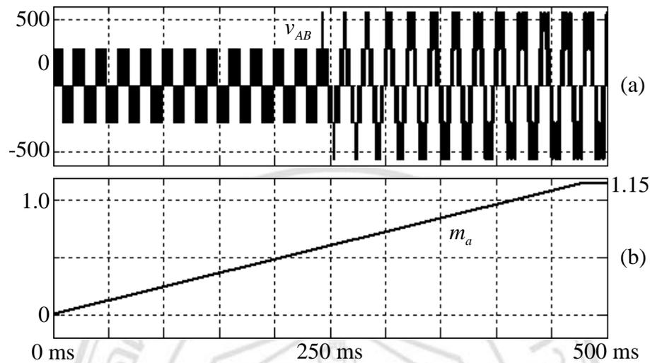
Figure 3.8 Simulation waveforms of dynamic response operation for a ramp modulation index reference (a) line-to-line voltage  $v_{AB}$  (b) modulation index  $m_a$ .
