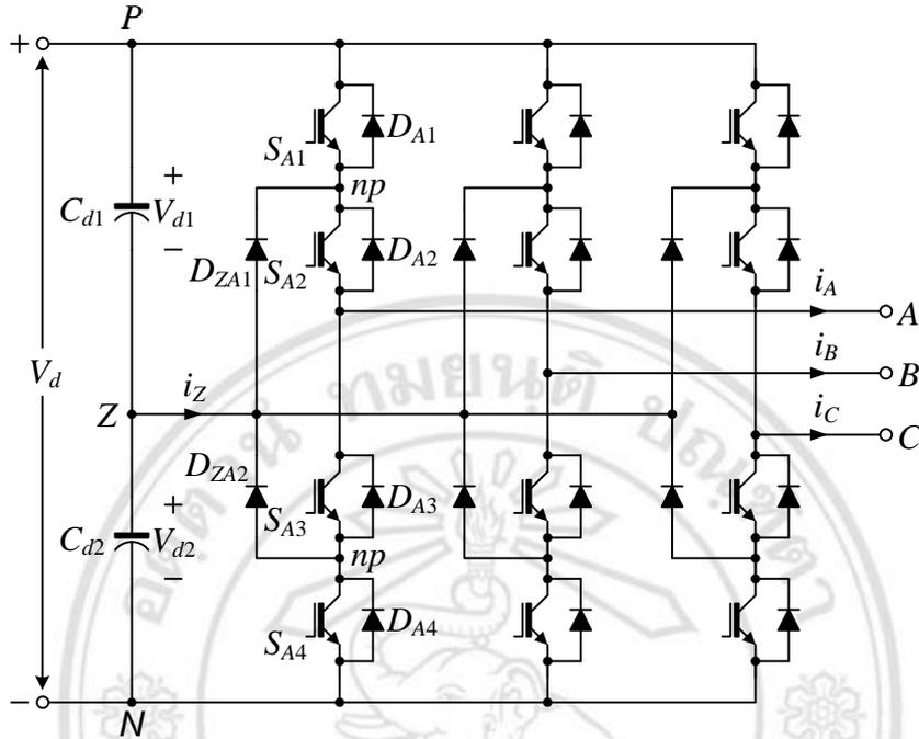
Figure 3.2 Simplified schematic of the power circuit of the three-level NPC VSI.
