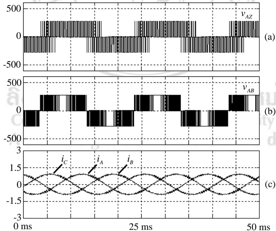
Figure 3.10 Simulation waveforms at low modulation index,  $m_a = 0.5$  (a) pole voltage
