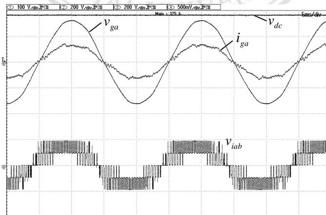
Figure 3.20 Experiment waveforms of the grid-side converter in the rectifying mode at unity power factor operation.
