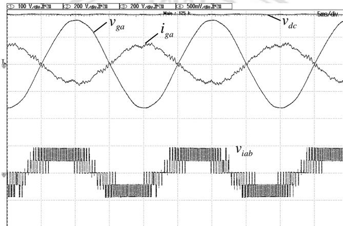
Figure 3.19 Experiment waveforms of the grid-side converter in the inverting mode at unity power factor operation.
