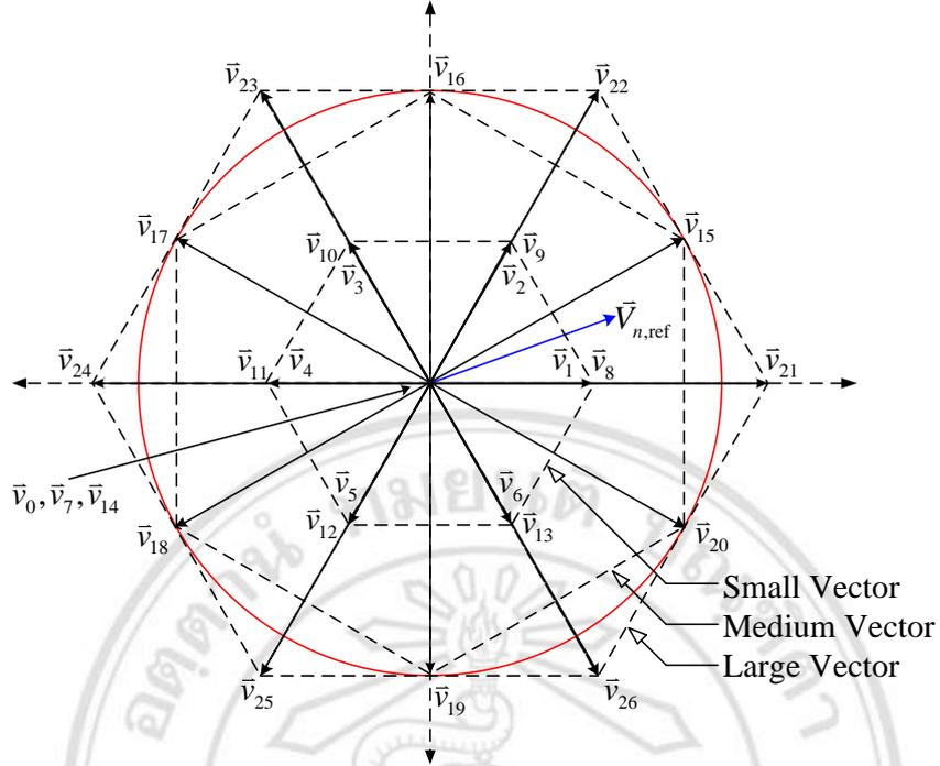
Figure 3.3 Space vector voltages diagram of the three-level NPC VSI.
