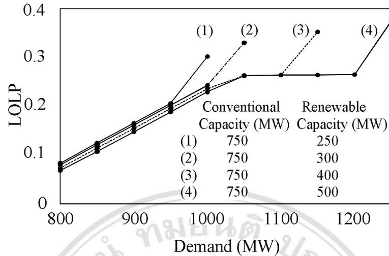
Figure 6.14 Comparison of LOLPs under various penetration levels of renewable energy resources.
