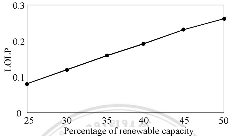
Figure 6.16 Impact of penetration level of renewable energy resources on LOLP.
