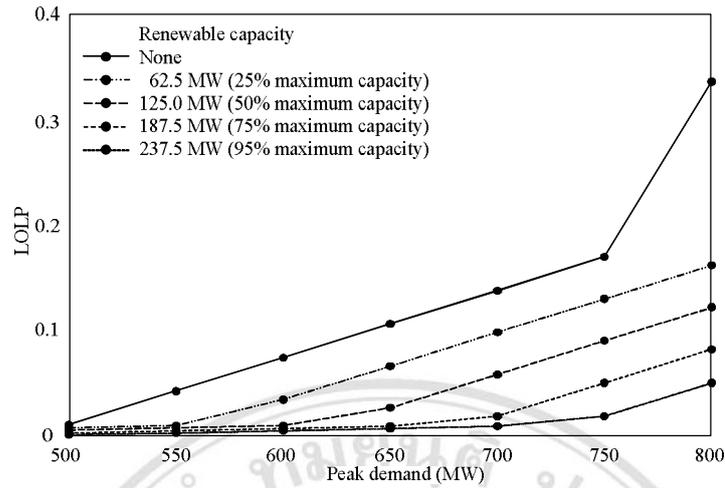
Figure 6.6 Comparison of loss of load probabilities under various generation capacities and peak-demand conditions.
