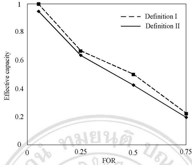
Figure 6.10 Effective capacity of renewable unit with 25-MW increment.
