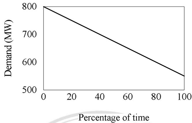
Figure 6.12 Load duration curve of the test system.
