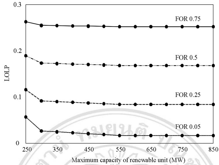
Figure 6.8 Comparison of loss of load probabilities under various maximum capacities and forced outage rates of the renewable unit.
