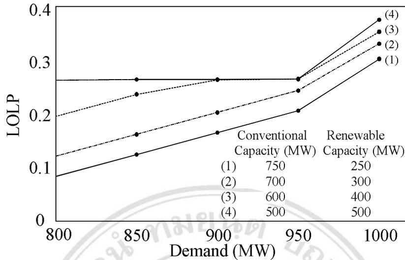
Figure 6.15 Comparison of LOLPs under various penetration levels of renewable energy resources with reduction of conventional resource.
