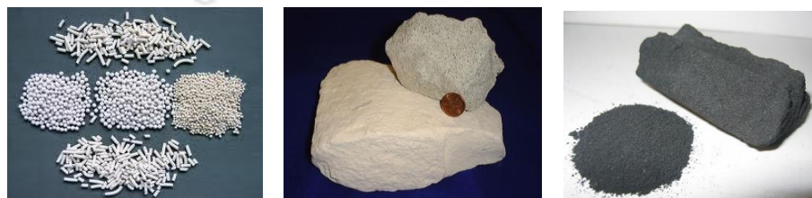
Figure 2.4 Molecular Sieve, Zeolite, and Activated Carbon [Molecular Sieve, Zeolite, and Activated Carbon 2015].
