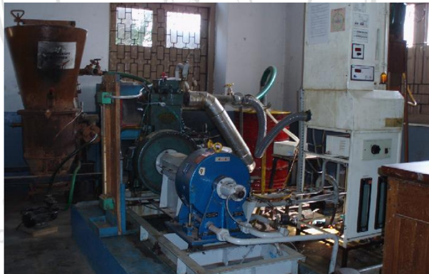
Figure 1.13 Overall view of 5.2 kW diesel engine on producer gas fueled (Banapurmath et al., 2008)
