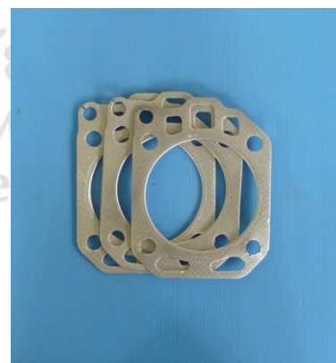
Figure 3.5 Gasket kit and special gasket of cylinder head in modified engine
