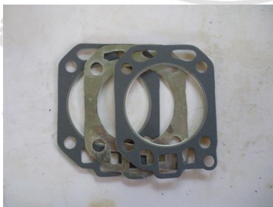
Figure 3.5 Gasket kit and special gasket of cylinder head in modified engine
