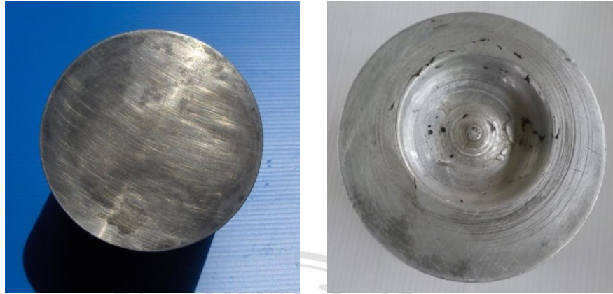
Figure 3.15 Piston crown of bath tub and cavity combustion chamber (9.7:1)
