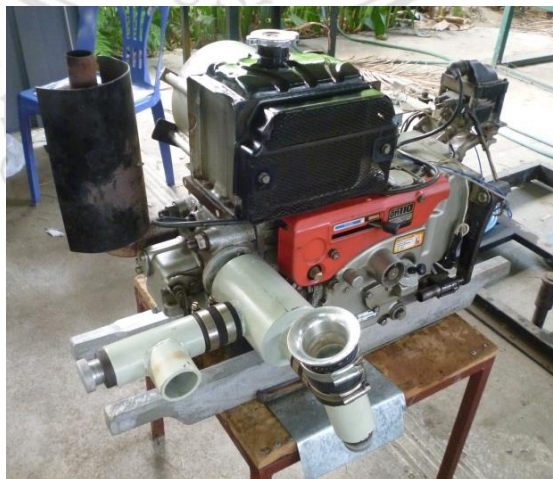
Figure 5.4 Gas engine after modified
