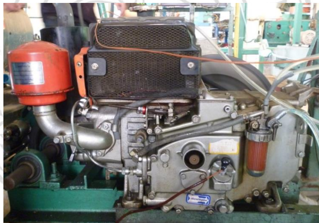
Figure 5.6 Diesel engine before converting to the gas engine
