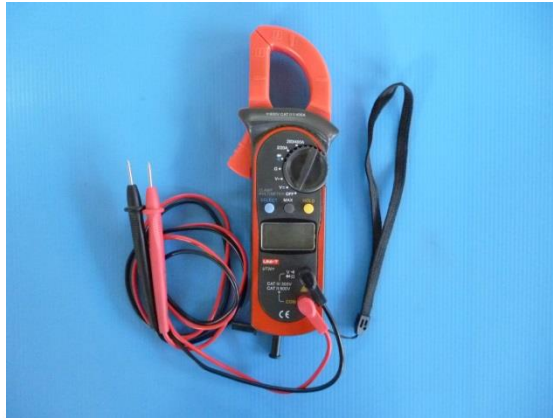
Figure 5.16 Multi meter use measures electrical load
