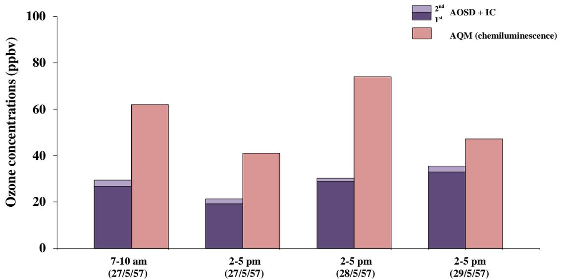
Figure 3.2 Comparison of 3-hr ozone concentrations of developed AOSD with reference values from the AQM
