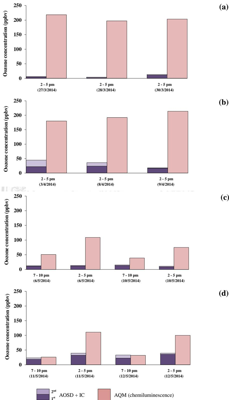
Figure 3.1 Ozone concentrations (3-hr) obtained from the same absorbing solution (0.1 %  $\text{NaNO}_2$ / 0.1 %  $\text{Na}_2\text{CO}_3$ / 1% ethylene glycol) with different air flow rates (L/min) (a) 2.0, (b) 1.5, (c) 1.0 and (d) 0.5
