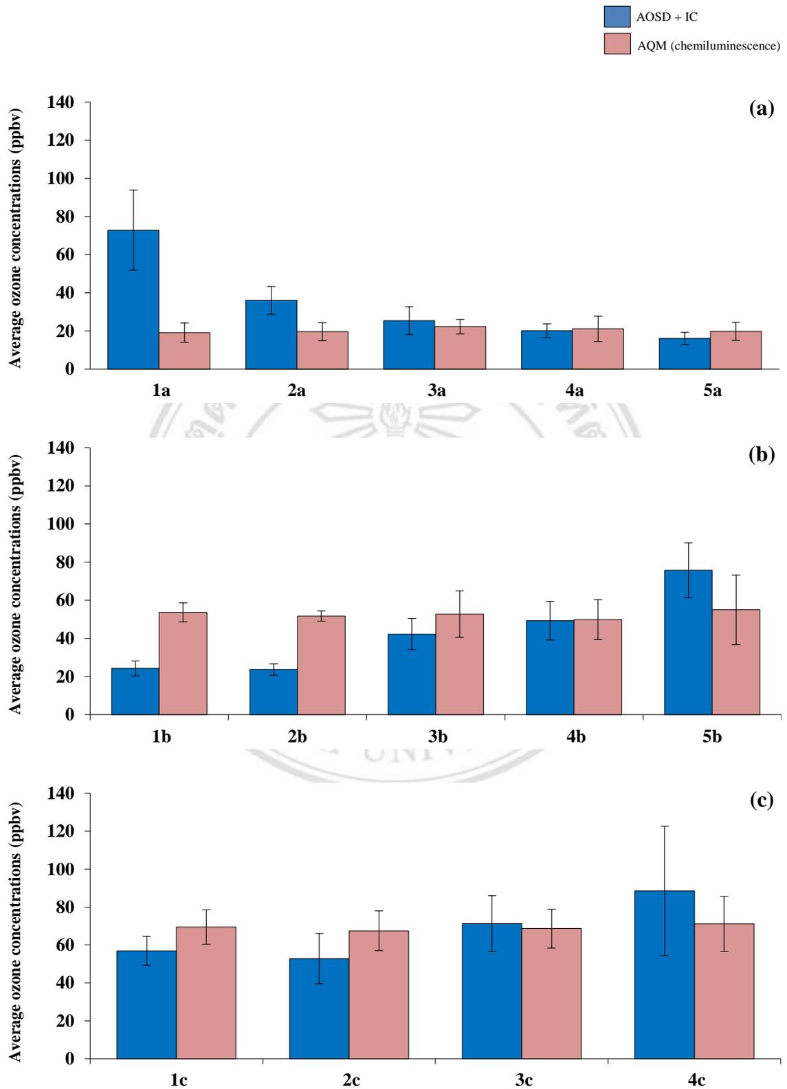
Figure 3.3 Average hourly ozone concentrations obtained from the developed AOSD at different sampling conditions and the reference values in (a) wet season (<35 ppbv), (b) dry season (30-70 ppbv) and (c) dry season (>70 ppbv)
