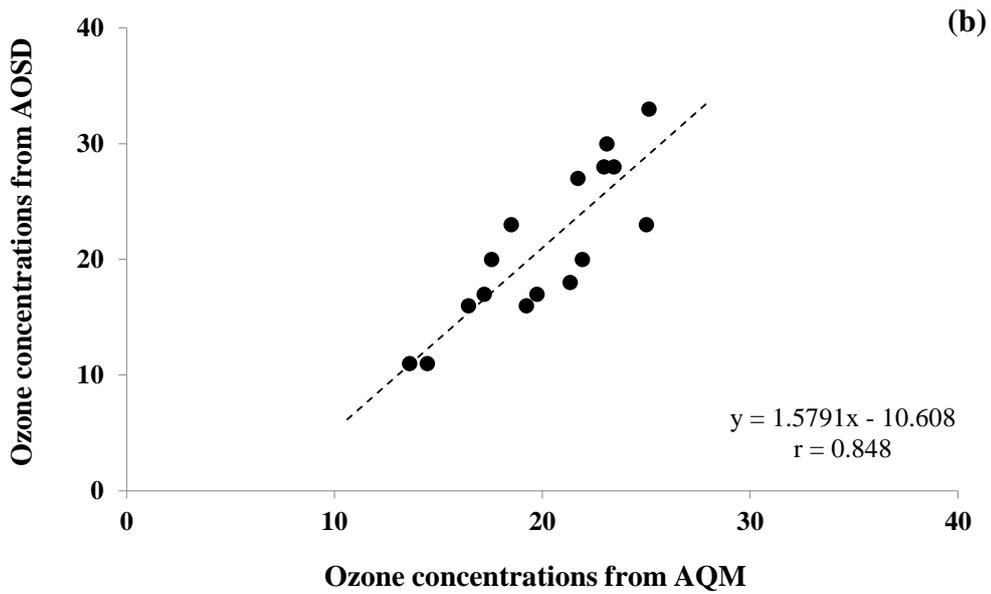
Figure 3.4 Hourly ozone concentrations in wet season (<35 ppbv) (a) Comparison of ozone obtained from AOSD and AQM (b) Correlation of ozone concentrations between AOSD and AQM
