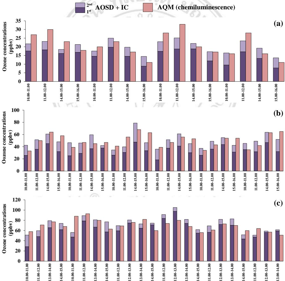
Figure 3.7 Comparison of 1-hr ozone concentrations obtained from the developed AOSD with reference values from the AQM under the optimum condition (a) Wet season (<35 ppbv), (b) Dry season (30-70 ppbv) and (c) Dry season (>70 ppbv)
