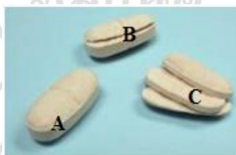
Figure 2.5: Comparative photo of complete tablet (A), capping tablet (B) and laminating tablet (C) (picture from http://www.pharmainfo.net/gate-quizzes/processing-problems-of-tablets ; accessed 7 Feb 2014)
