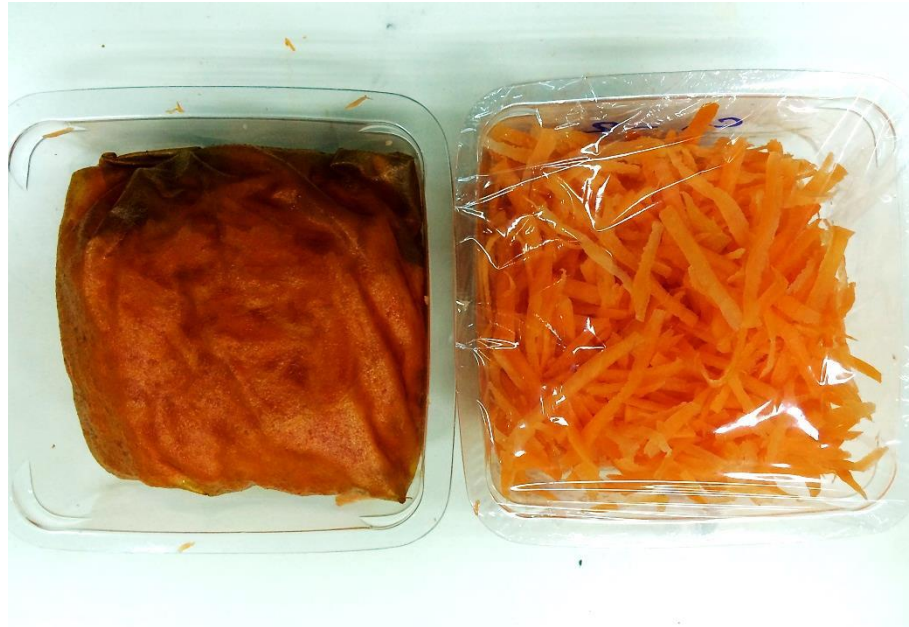
Figure A-5 Shelf life testing of fresh cut carrot: Coffee pulp film (left); Conventional packaging; polyvinylchloride cling film (right)
