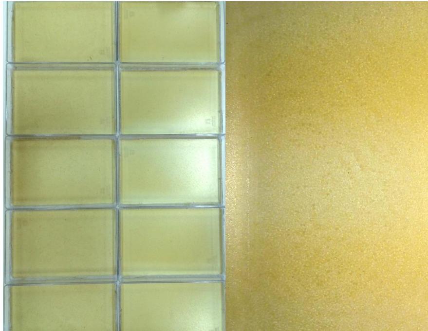
Figure A-3 Coffee pulp film during drying process (left) and final formulation of coffee pulp film (right)
