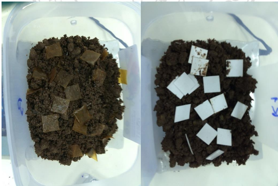
Figure A-4 Biodegradability testing: Coffee pulp film (left); Control (right)
