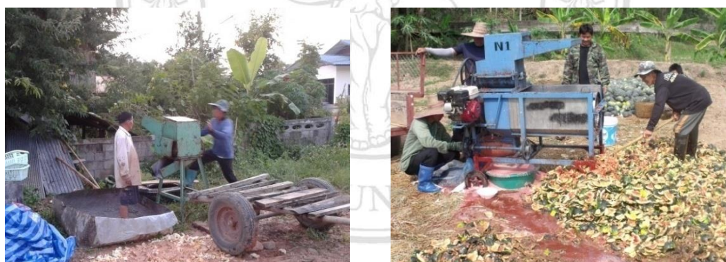
Figure 3.25 Mill machines for vegetable seed harvest provided by seed companies for cucumber (left) and for watermelon (right)
