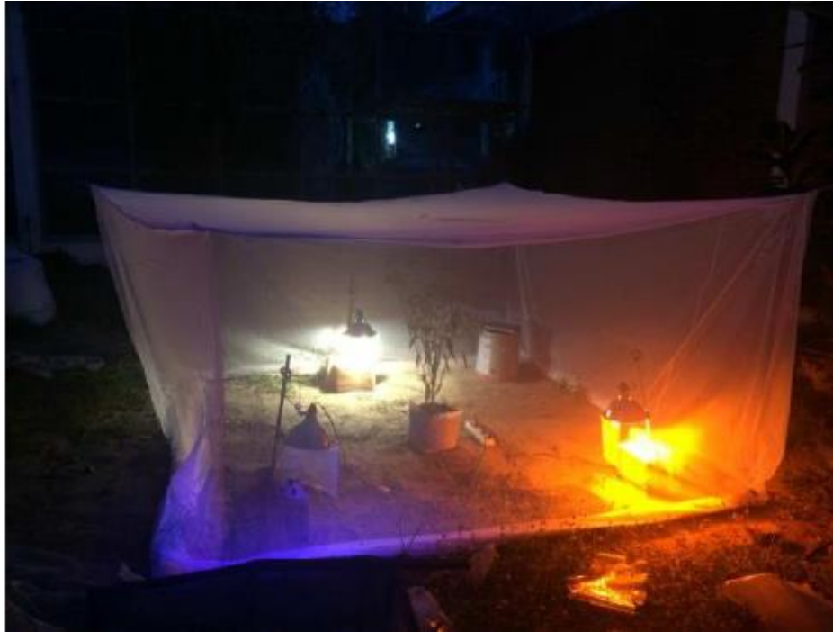
Figure3.4e. Multiple choice experiments with three different lighting treatments (UV light, Warm White and Yellow light) under outside conditions)
