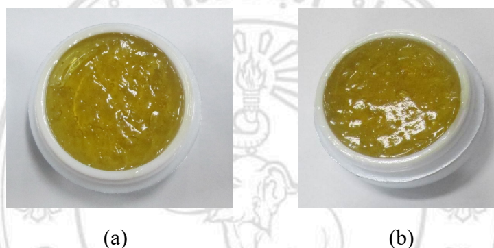
Figure 4.17 The algal gel product (a) and algal gel after 6 cycles of heating-cooling (b)
