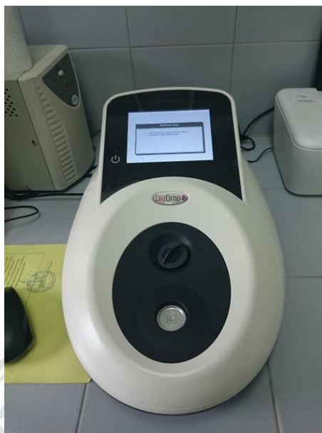
Figure.3.11. Photograph of BioDrop TOUCH, the gray circle is a direct micro-volume sample port
