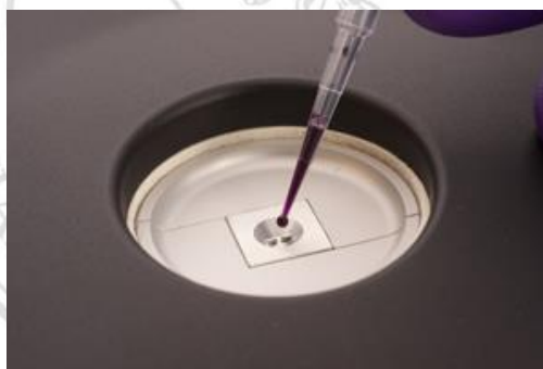
Figure.3.12. Dropping area for measuring naked DNA concentration is stand on middle of Bio-drop spectrophotometer, which is a small shallow pit.
