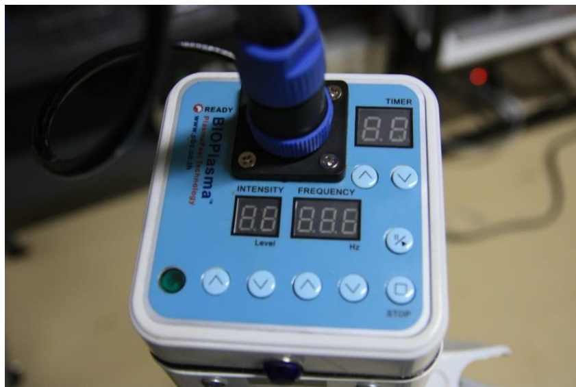
Figure.3.2. The CAPPJ apparatus used in the experiment. A photograph of the control panel's interface is at the top systems. It allows adjusting intensity and frequency of the plasma output.
