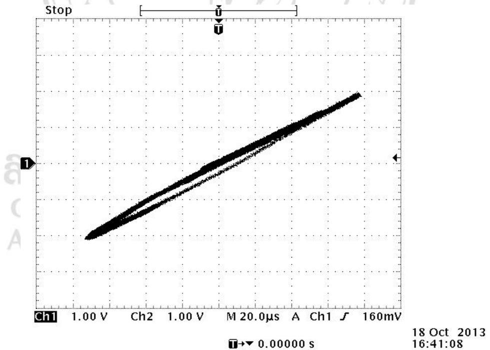
Figure.4.6. Lissajous graph was measured by using the condition of intensity level 5 and frequency 110 Hz
