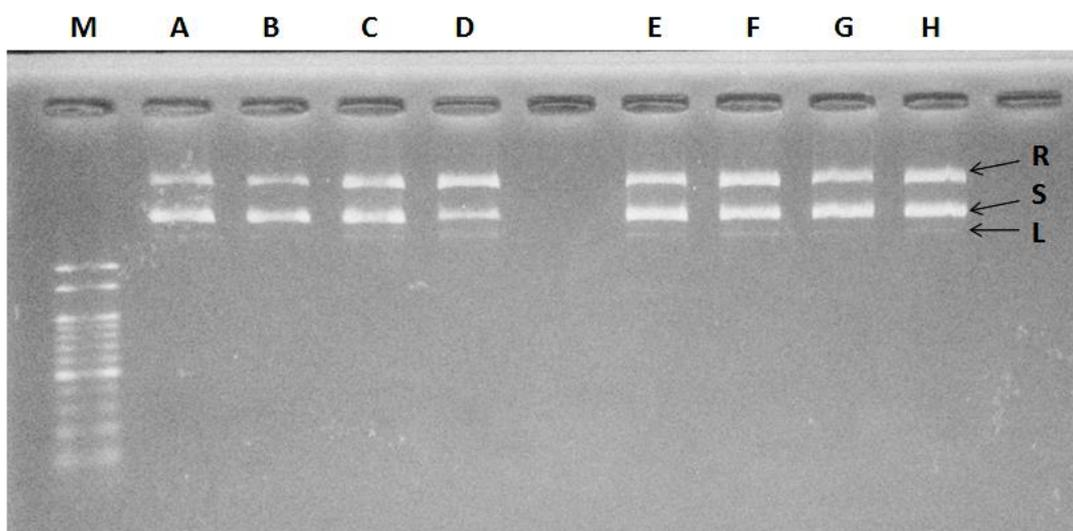
Figure.4.18. Electrophoresis result for comparison. M: Marker. A and E: I1/50Hz, dry. B and F: I1/50Hz, wet. C and G: I5/50, dry. D and H: I5/50Hz, wet. A-D: without electrical field. E-H: with electrical field. R: relaxed form. S: supercoiled form. L: linear form.
