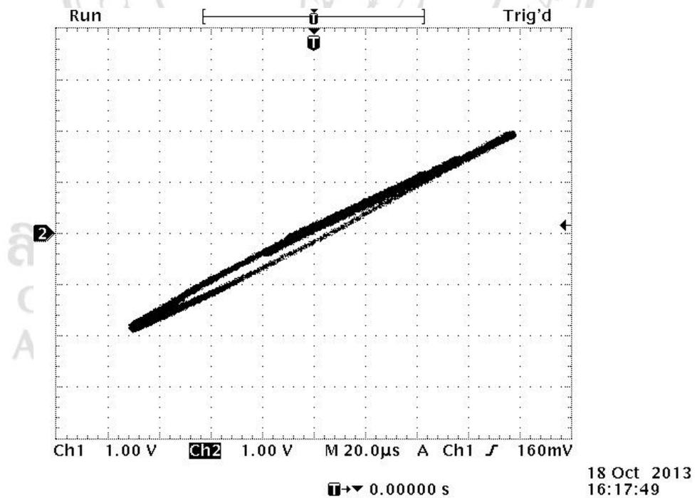
Figure.4.8. Lissajous graph was measured by using the condition of intensity level 10 and frequency 50 Hz
