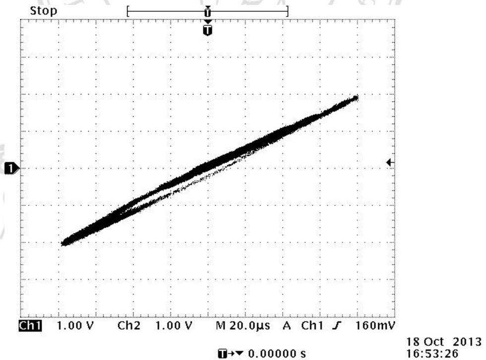
Figure.4.4. Lissajous graph was measured by using the condition of intensity level 5 and frequency 10 Hz
