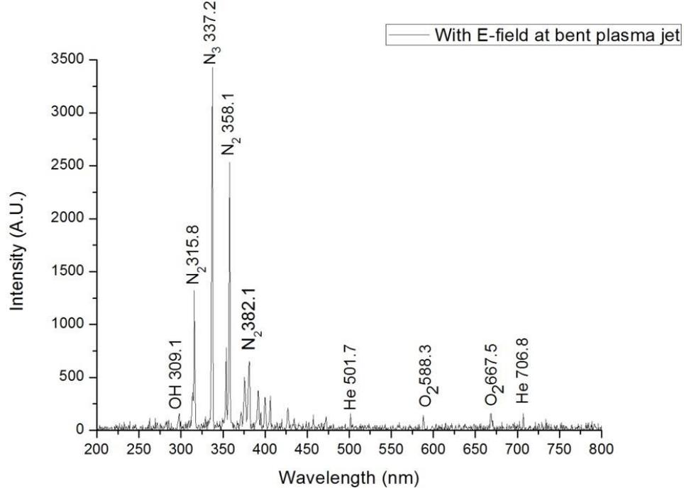
Figure.4.15. Optical emission spectra (OES) of the CAPPJ, OES detect from the bent plasma jet after it traversed the electrical field
