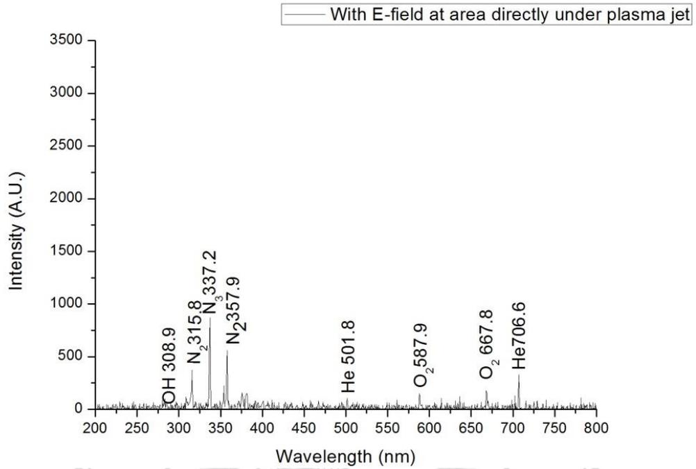
Figure.4.14 Optical emission spectra (OES) of the CAPPJ, OES detect from the area directly under the plasma jet exit, where the main part of the original plasma jet was bent away after it traversed the electrical field.
