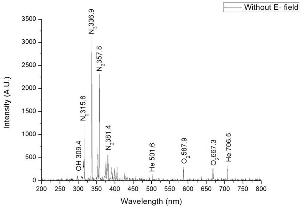
Figure.4.13. Optical emission spectra (OES) of the CAPPJ, OES detect from the original plasma jet.
