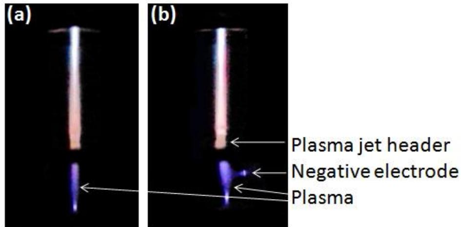
Figure.4.12. Photograph of the plasma jet when it traverses a pair of parallel electrodes when the electrical field is (a) off and (b) on
