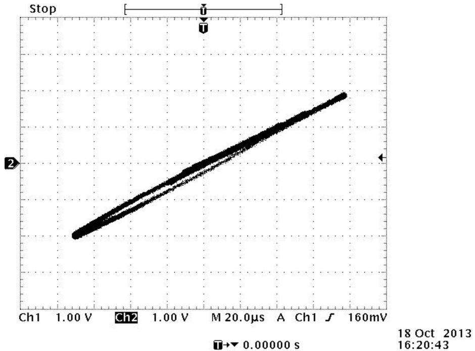
Figure.4.9. Lissajous graph was measured by using the condition of intensity level 10 and frequency 110 Hz
