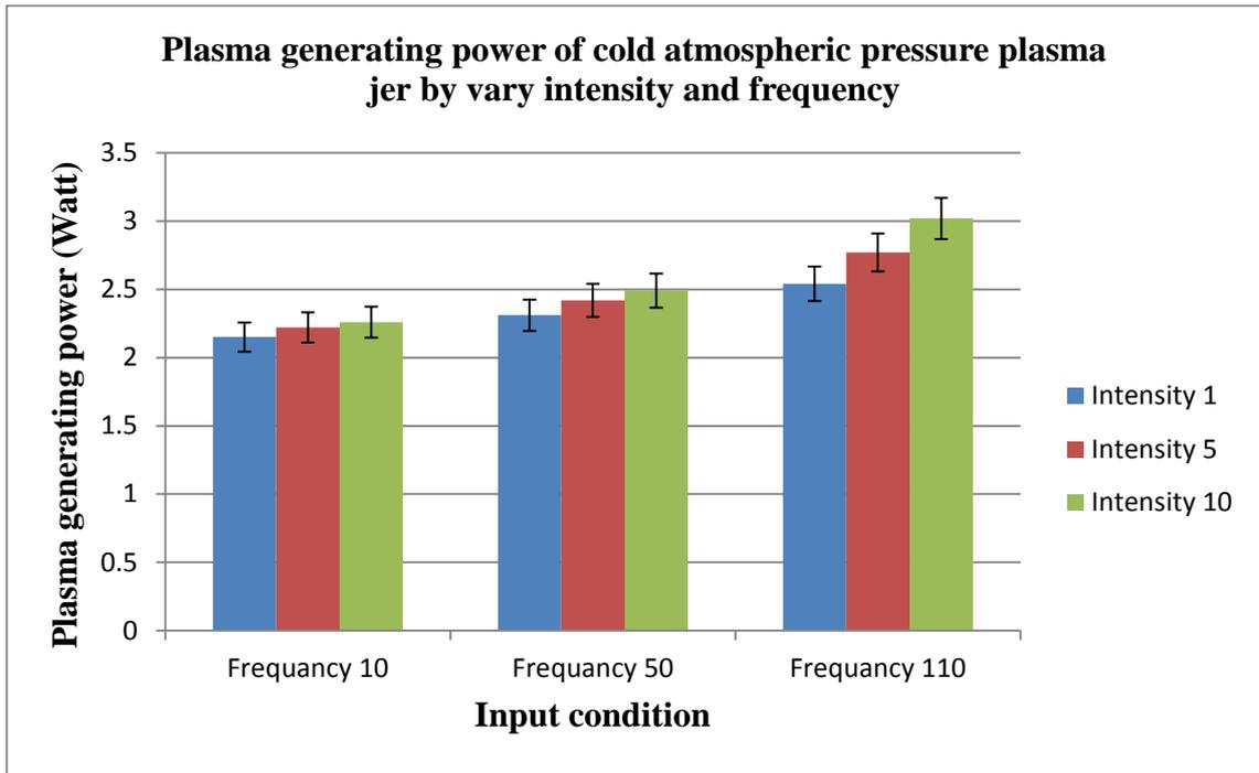
Figure.4.11. Graph of measured plasma generating power, as a function of control parameter combinations of intensity in I number and frequency in Hz, i.e. I/Hz.
