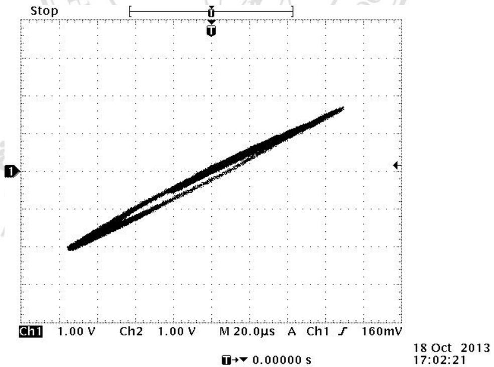
Figure 4.2. Lissajous graph was measured by using the condition of intensity level 1 and frequency 50 Hz
