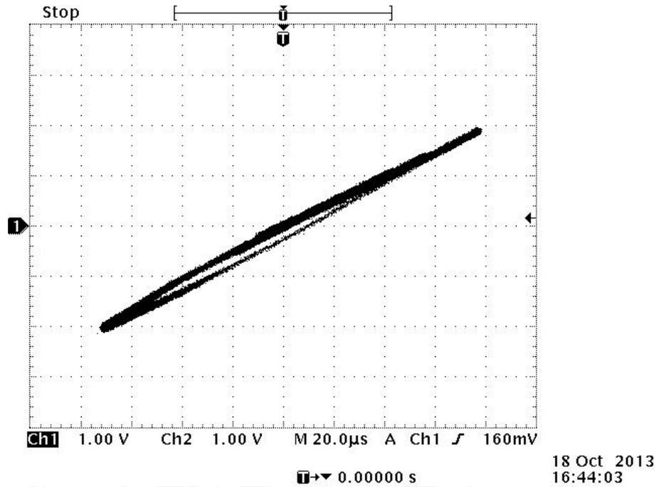
Figure. 4.5. Lissajous graph was measured by using the condition of intensity level 5 and frequency 50 Hz
