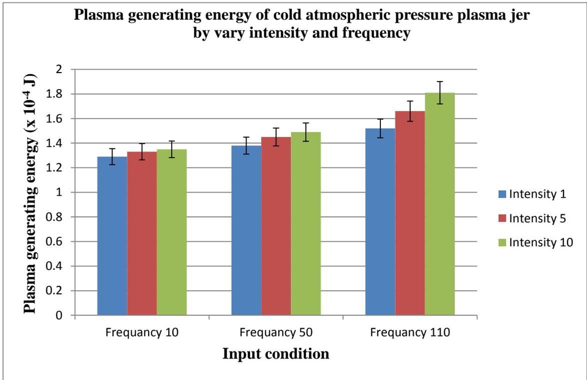
Figure.4.10. Graph of measured plasma generating energy, as a function of control parameter combinations of intensity in I number and frequency in Hz, i.e. I/Hz.
