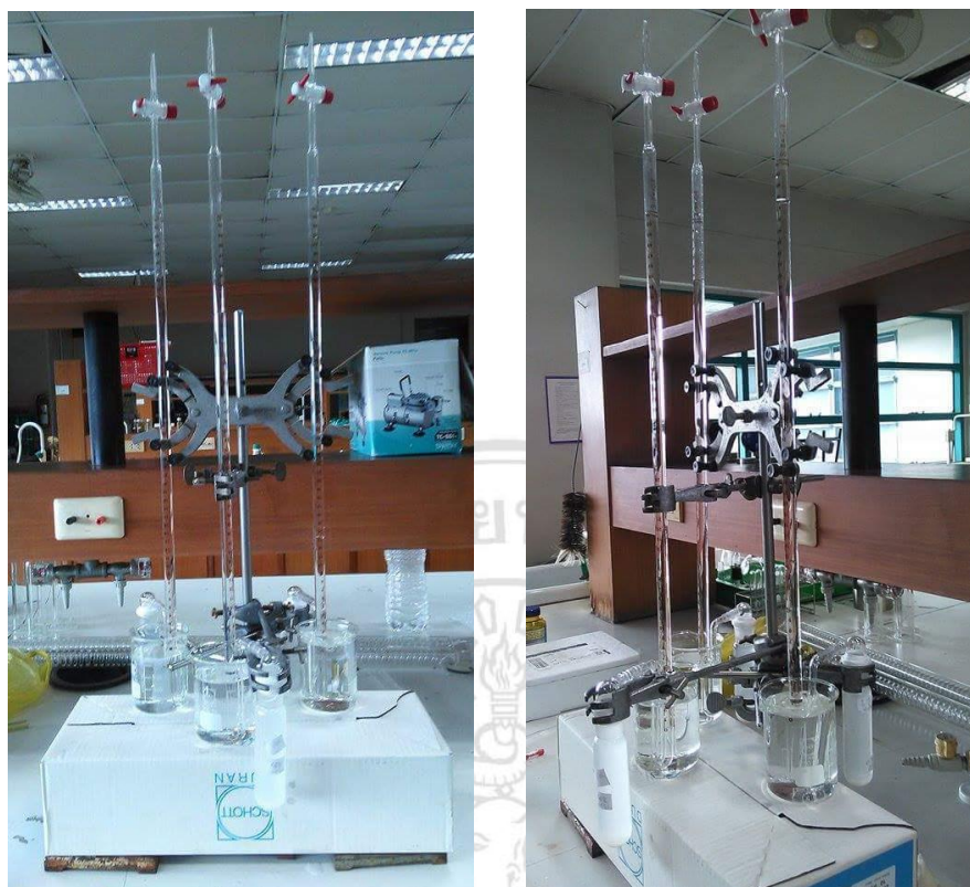
Figure 4. Apparatus in the experiment of oxygen releasing.
