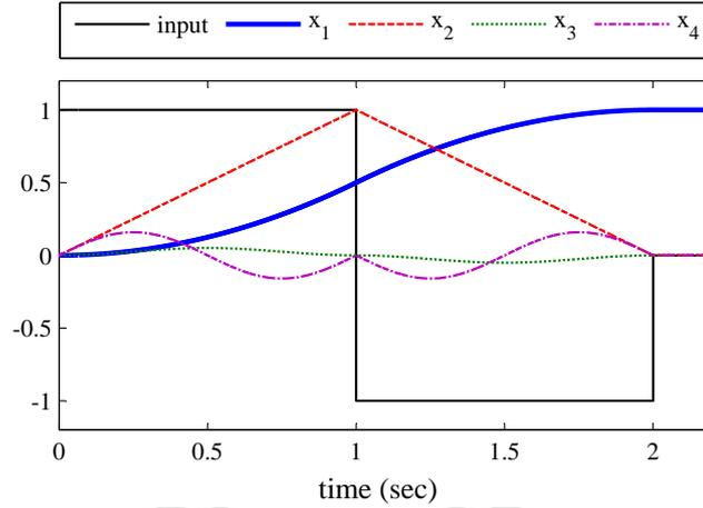
Figure 4.1: Time-optimal motion of undamped flexible structure
