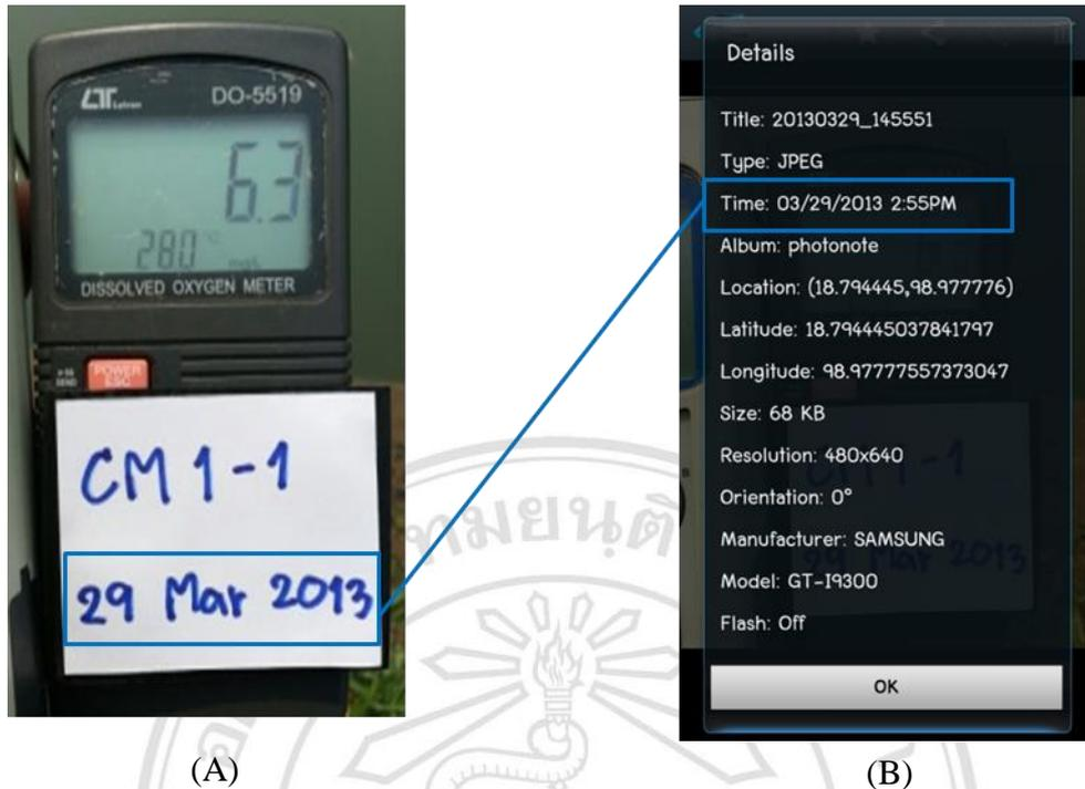
Figure 2.4 (A) A label showing name of sampling site (such as CM 1-1) and date of measurement (such as 29 Mar 2013), (B) Data on a photo file showing date, time, geographic coordinate and details of photo (see text)
