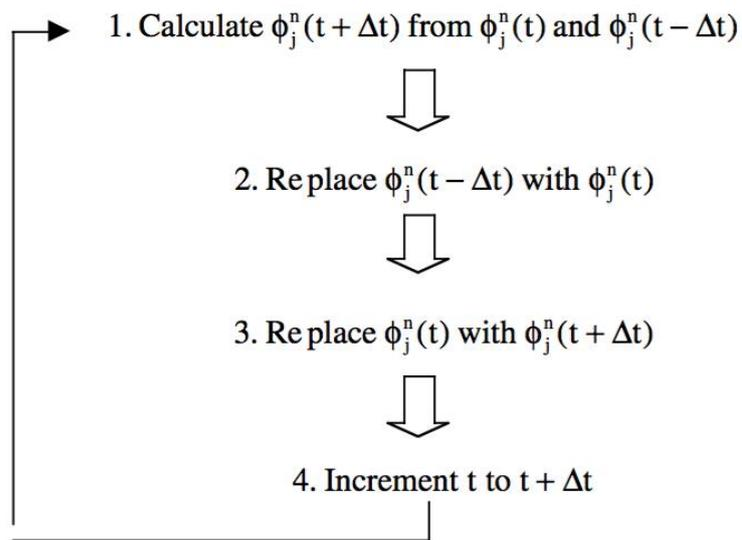
Figure 2.3: Time stepping Finite difference workflow (Youzwishen et al, 1999).
