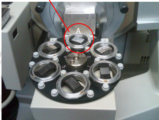
Figure 3.6 Rikaku TTRAXIII X-ray diffractometer. Diffraction pattern can be obtained if the orientation of sample satisfied Bragg's law.
