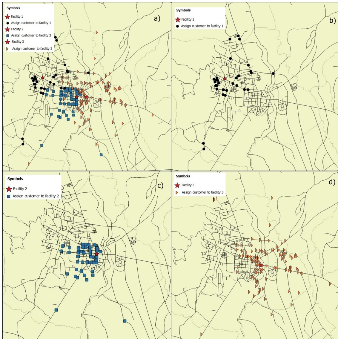
Figure 4.12: The 200 node network optimal solution after size reduction with nodes of degree 1 and 2 removed. a) 3 facilities and client groups b) client groups of facility 1 c) client groups of facility 2 d) client groups of facility 3.
