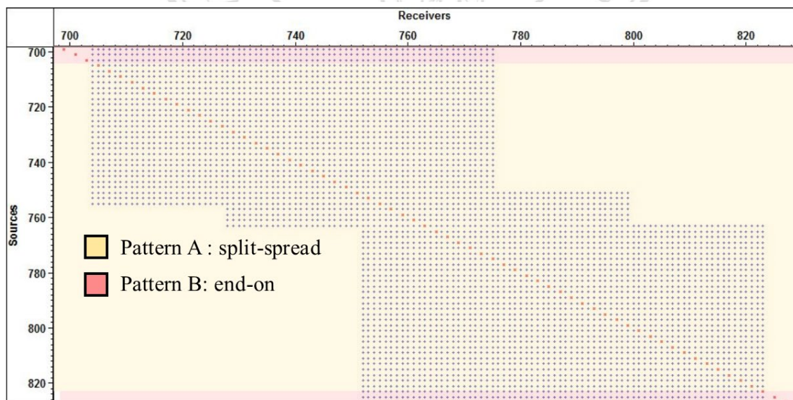
Figure 2.16 shows stacking chart of survey Line MO-3 (red and blue dots are shot and receiver locations) with split-spread configuration (yellow zone) and end-on configuration (light-red zone).
