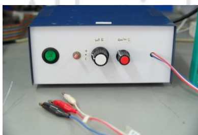
Figure 5.4 Home-made amperometric detector
