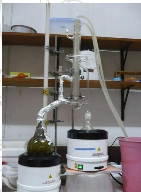
Figure 2.1 A modified Likens-Nickerson apparatus
