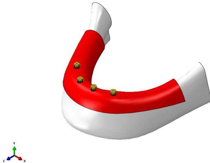
Figure 3.18 Edentulous mandibular with 4 mini dental implants at incisor and canine area (group7)
