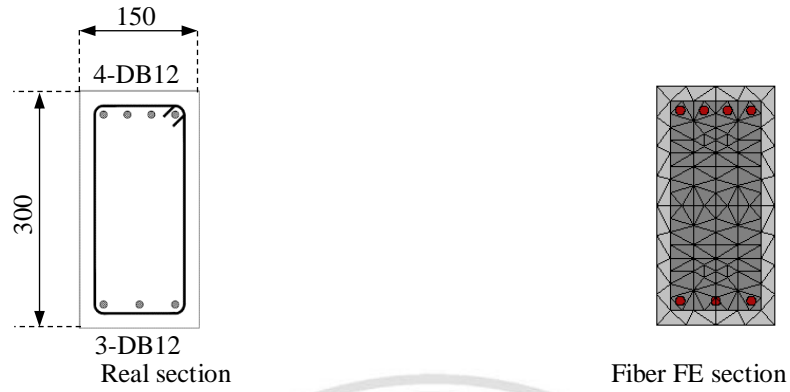
(a) RC beam of M1 specimen
