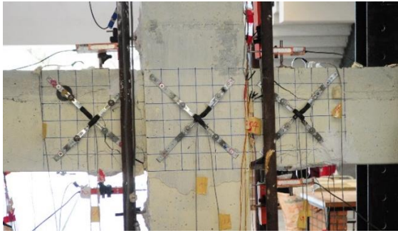
(d) Installing PI-gauges for measuring deformation at joint and beams
