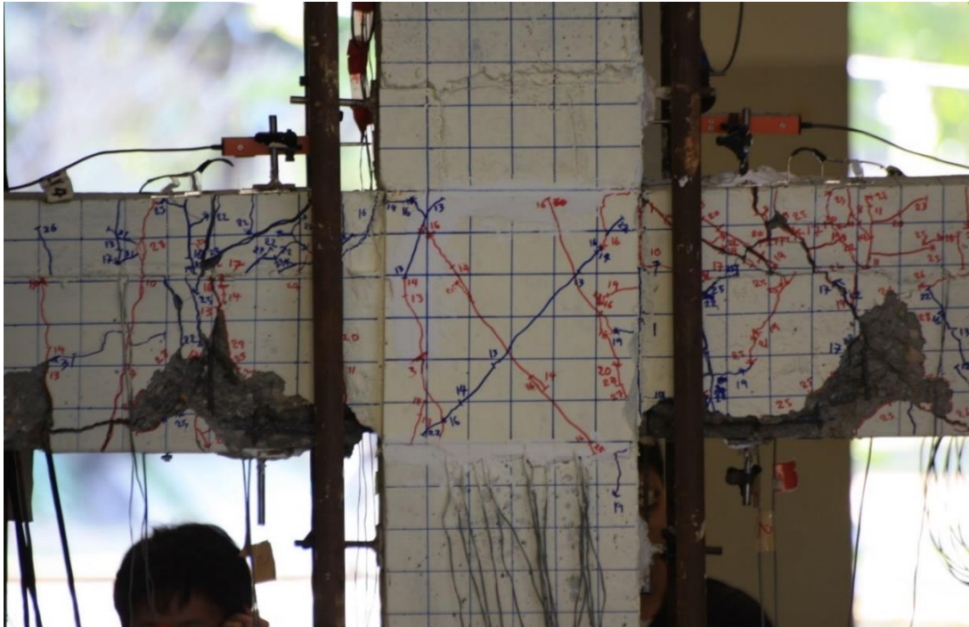
Figure 4.15 Damage level of specimen P5 at 3.50 percent story drift
