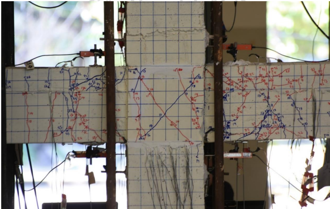
Figure 4.14 Crack distribution of specimen P5 at 1.75 percent story drift
