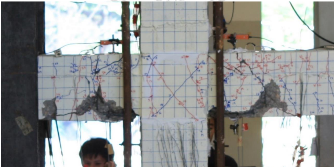
Figure 5.6 Crack distribution of precast specimen P5 at the end of testing
