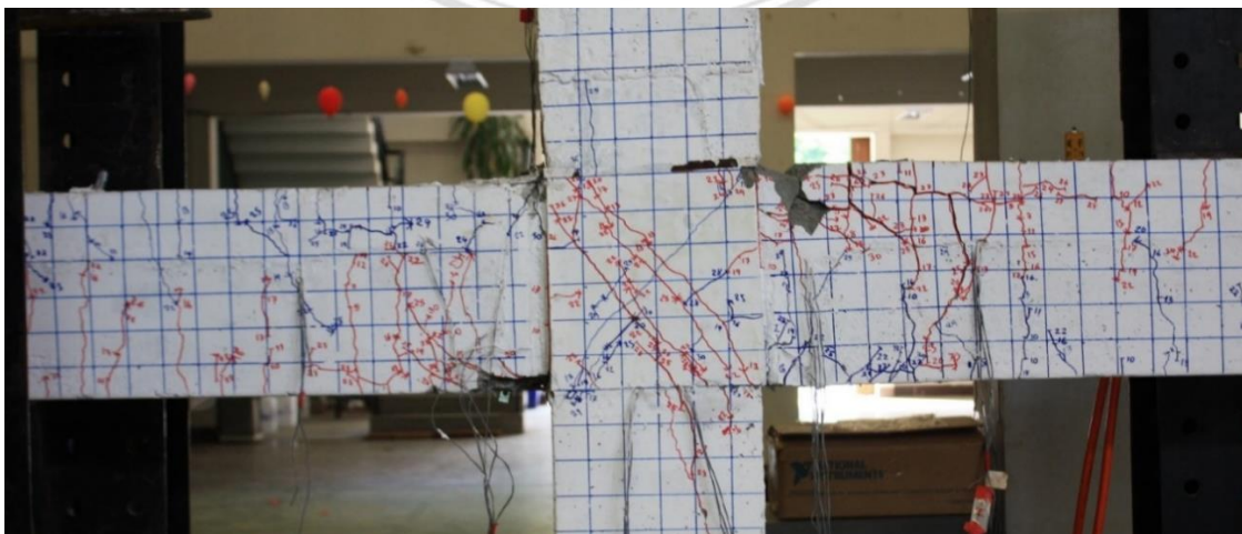
Figure 5.3 Crack distribution of precast specimen P2 at the end of testing
