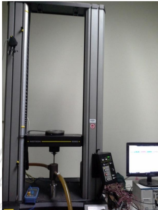
Figure 6.1: Compression test of densify plastic wastes and corn stover mixed in Instron machine.
