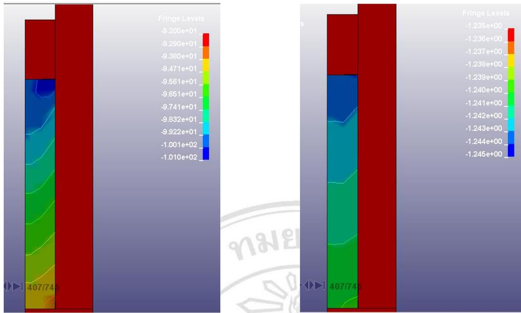
Figure 7.5: Distribution of compressive stress (left) and density (right) at 100 MPa.
