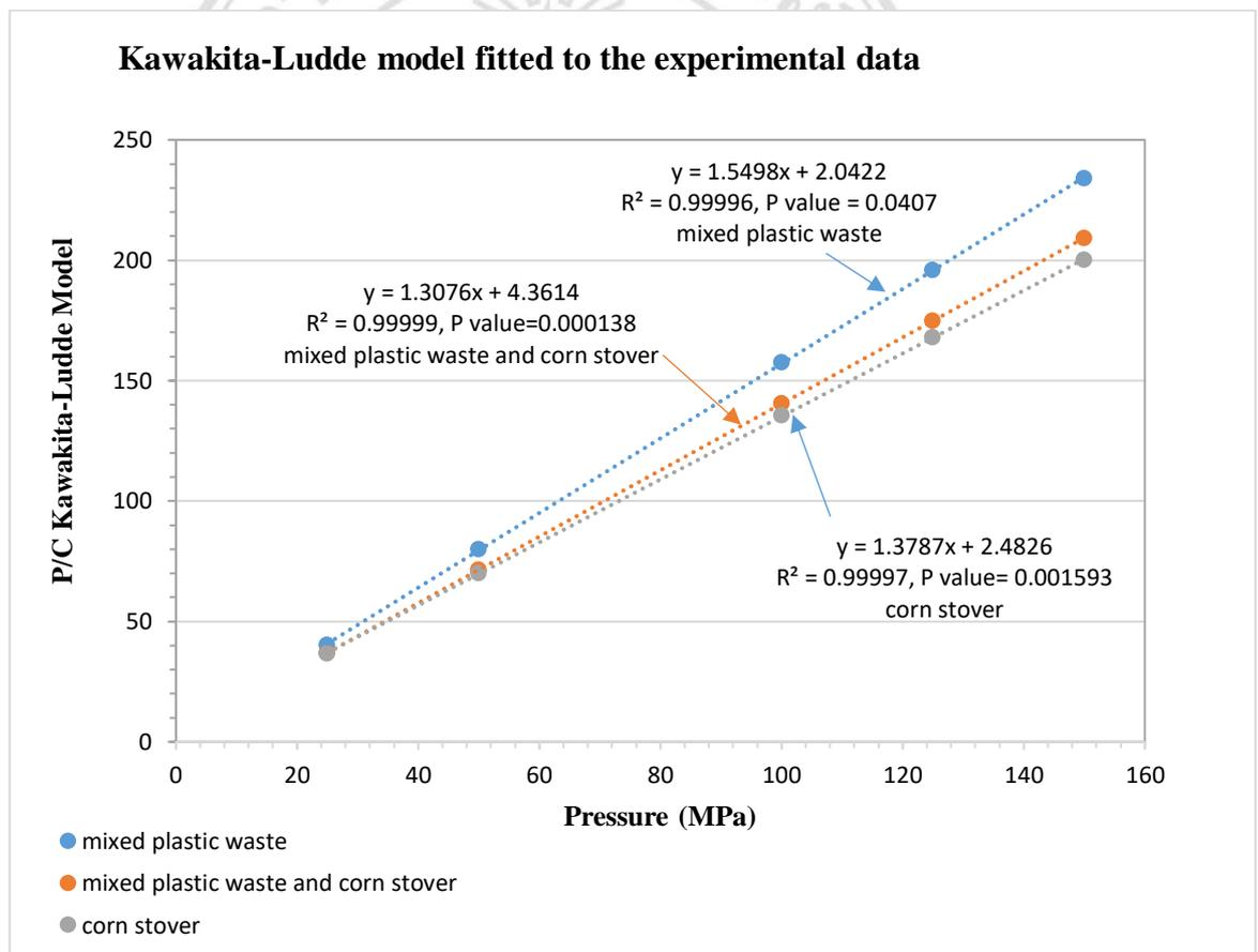
Fig. 7.1: The relation of P/C versus P fitted to the experiment data which obtained from Kawakita-Ludde model
