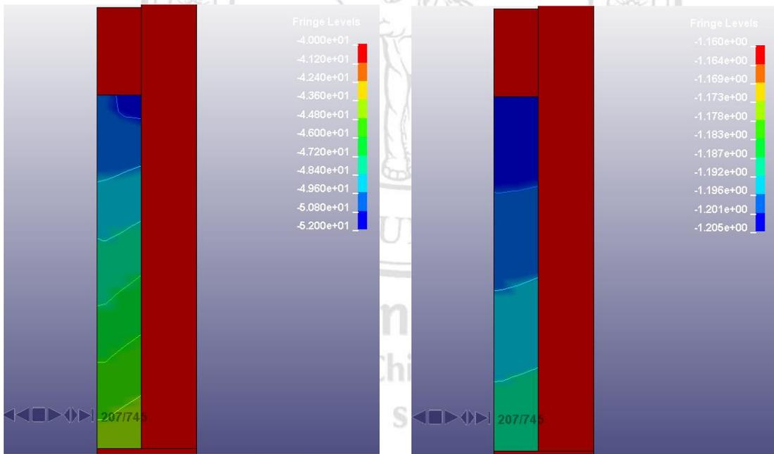
Figure 7.4: Distribution of compressive stress (left) and density (right) at 50 MPa.
