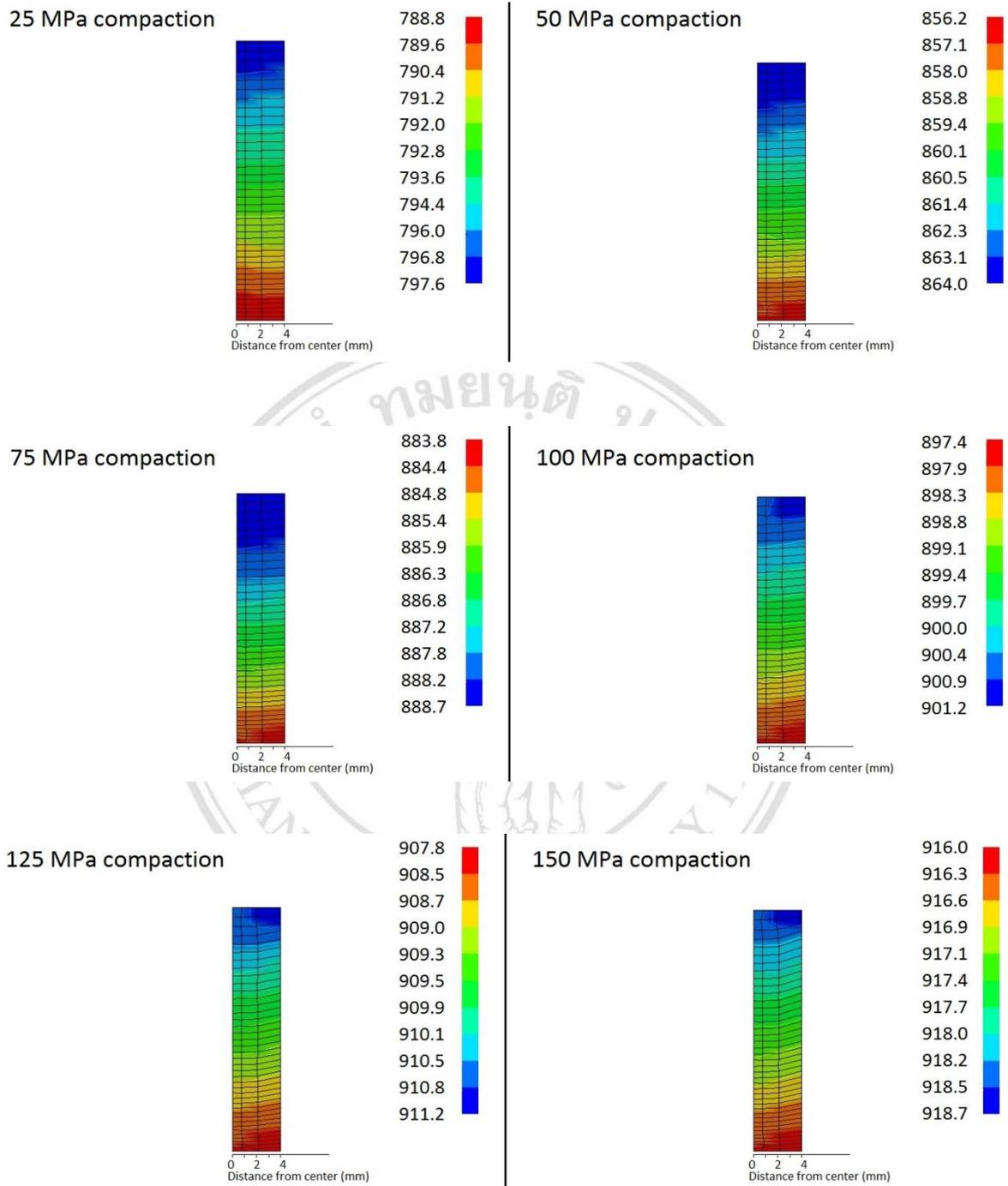
Figure 7.7: Density contour plots for 25, 50, 75, 100, 125 and 150 MPa.
