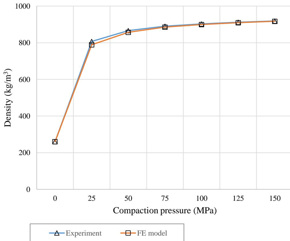
Figure 7.8: Comparison of density from FE simulation to experimental data.
