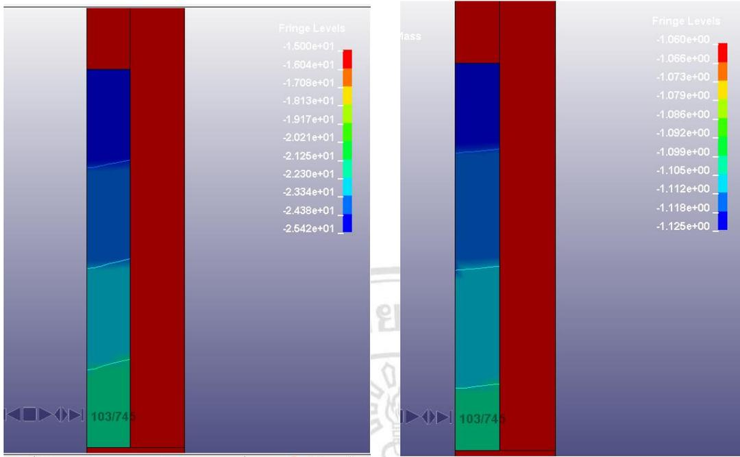
Figure 7.3: Distribution of compressive stress (left) and density (right) at 25 MPa.
