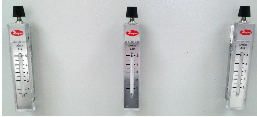
Figure 3.26 Flow meter and control.
