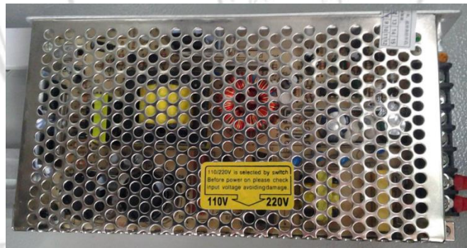
Figure 3.28 DC switching power supply 220VAC 50Hz/15VDC 20A.
