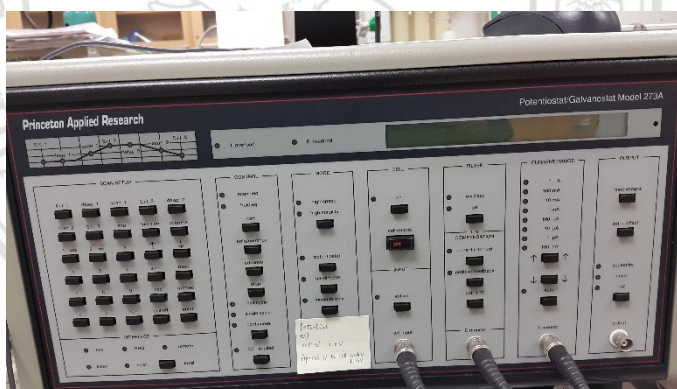
Figure 4.1 CV testing by Princeton Applied Research potentiostat/galvanostat model 263A
