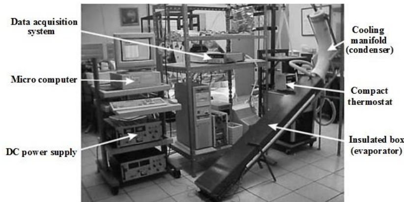
Figure 1.1 Experimental set up of the two-phase thermosyphon for solar domestic hot water system (Abreu & Colle, 2004)
