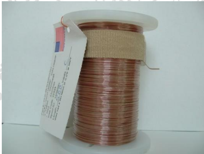
Figure 3.2 Thermocouple chromel-alumel (K-Type)
