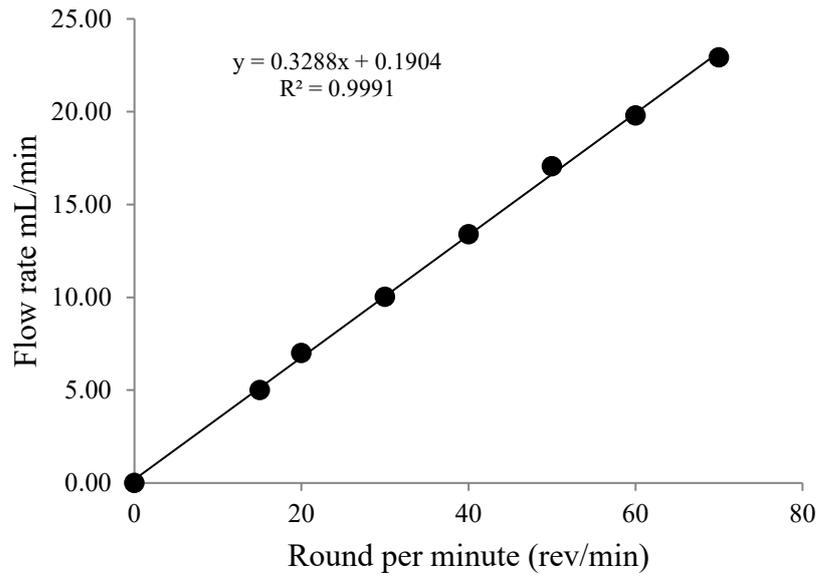
Figure 3.2 : Calibration curve for determine the flow rate
