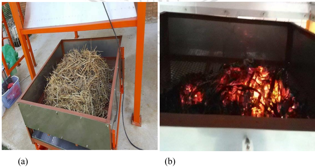
Figure 2.4 Open burning simulation, (a) dried biomass in burning tray, and (b) burning process.
