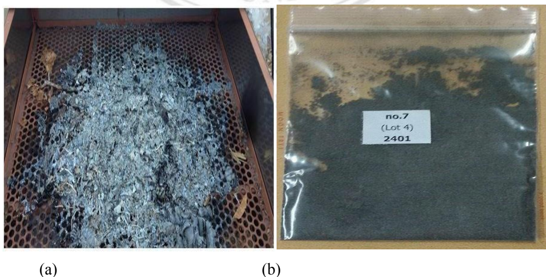
Figure 2.7 Ash sampling after open burning, (a) ash remained in the burning tray of the chamber, and (b) Sieved and packed ash samples (Chantara et al., 2017).
