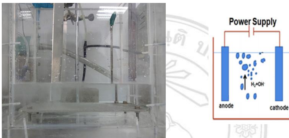
Figure 3.2 Micro bubbles generation by electro-flotation method
