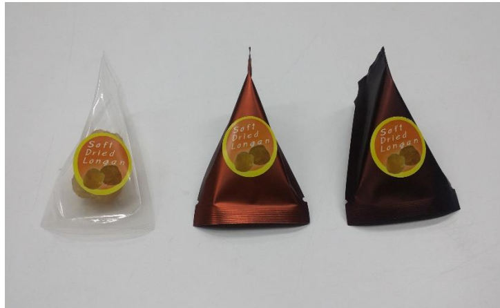
Fig. A – 7 Intermediate moisture longan packed in 3 different types of plastic bag (clear plastic bag, Aluminum bag with nitrogen and Aluminum bag without nitrogen).
