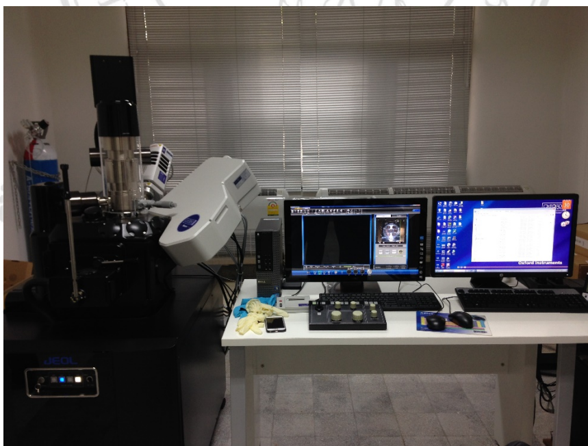
Figure A-4 Instrument image of scanning electron microscope (SEM) used in this study
