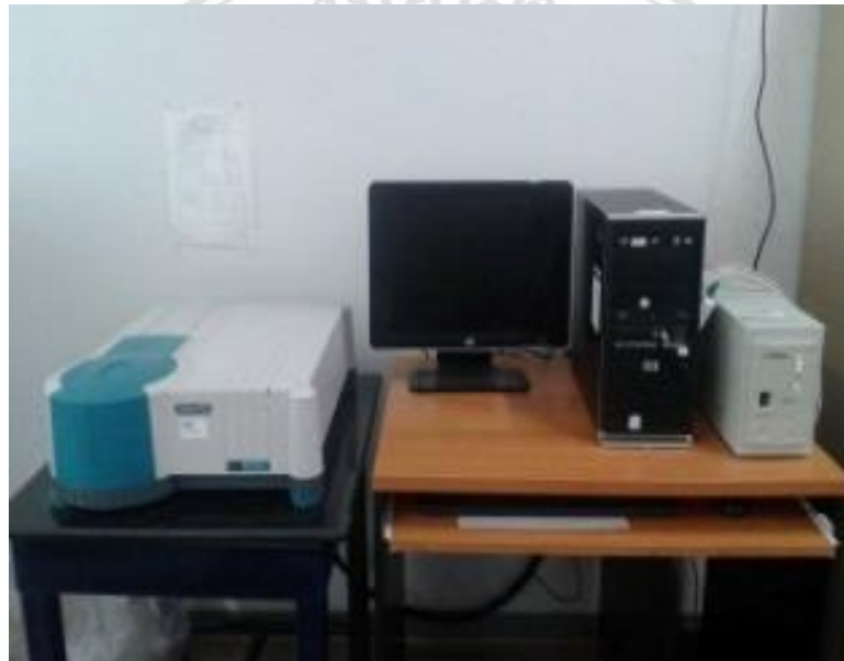
Figure 3.9 UV-vis spectrophotometer (Varian Cary 50, U.S.A).
