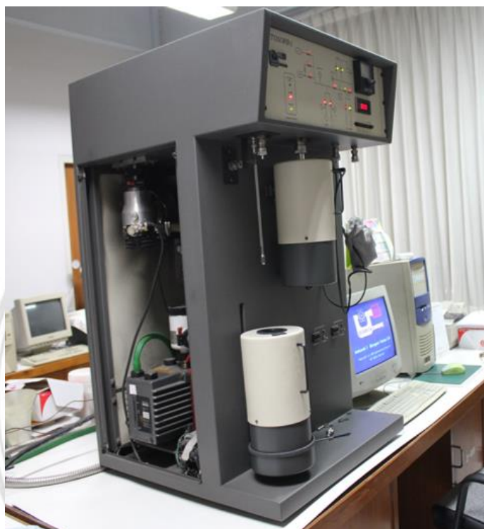
Figure 3.10 Brunauer-Emmett-Teller (Autosorb 1 MP, Quantachrome, USA)
