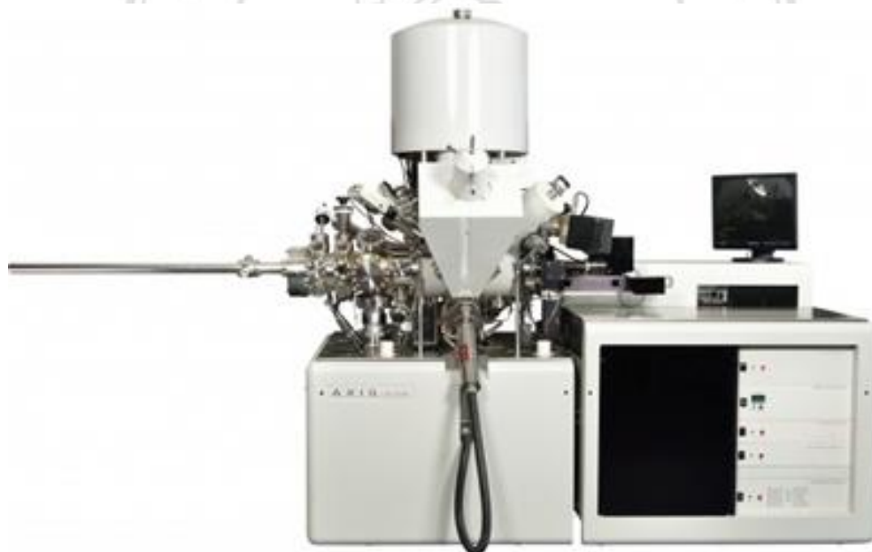
Figure 3.12 X-ray photoelectron spectroscopy (AXIS Ultra DLD, England)
