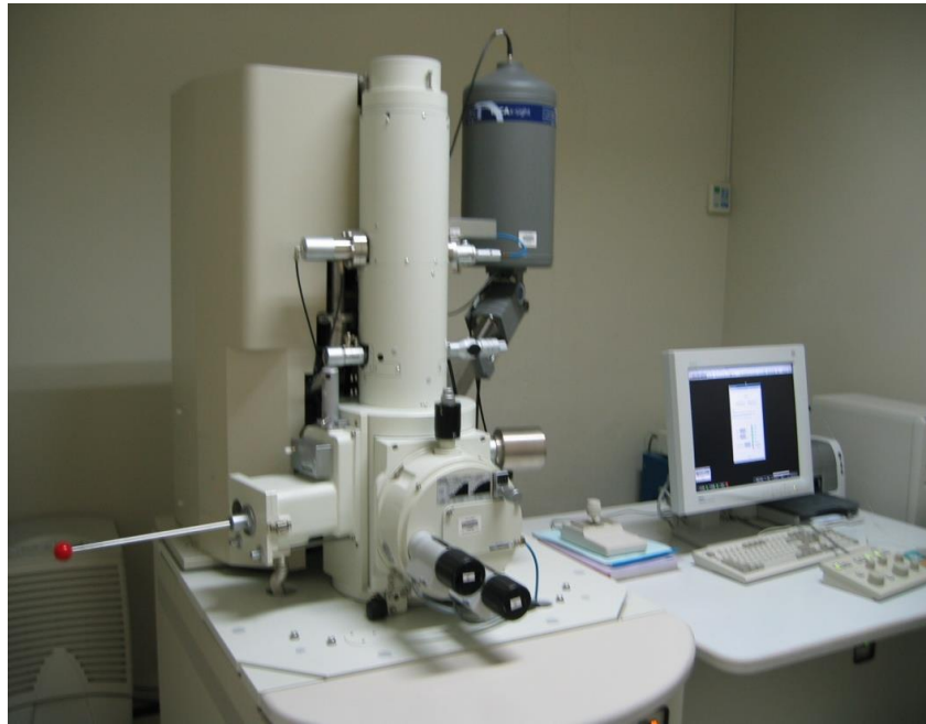
Figure 3.4 Field Emission Scanning Electron Microscope (FE-SEM, JEOL JSM-6335F) including Energy Dispersive X-ray Spectroscopy (EDS).
