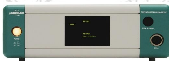
Figure 3.13 The \mu -Autolab Type III electrochemical work station (ECO-Chemie, Metrohm, Switzerland).
