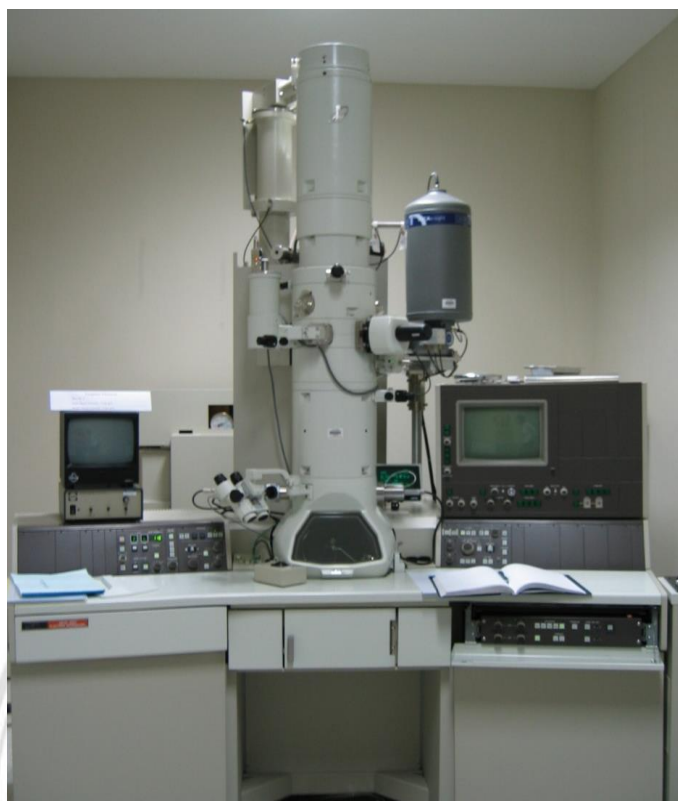
Figure 3.6 Transmission Electron Microscope (TEM, JEOL JEM-2010).
