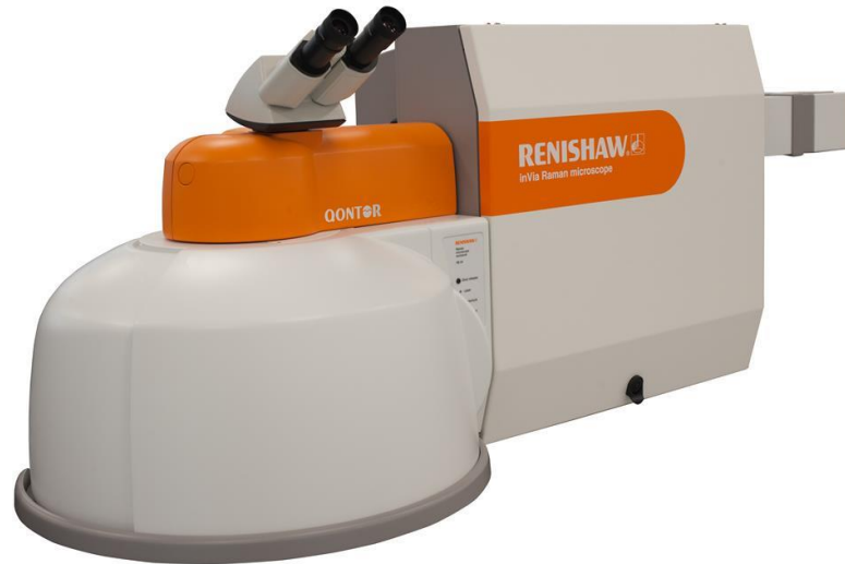
Figure 3.7 Raman spectrophotometer (Renishaw model Invia) operated with an argon ion laser.
