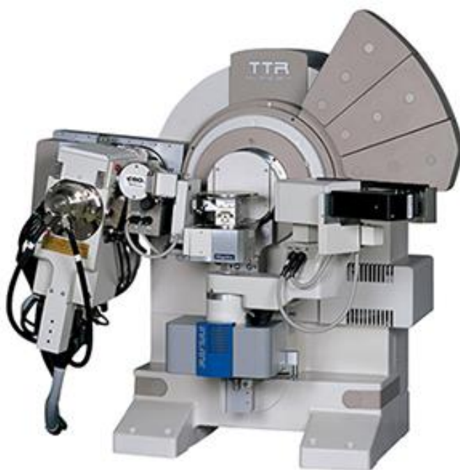
Figure 3.11 X-ray diffraction (GIXRD, Rigaku Ttrax III).
