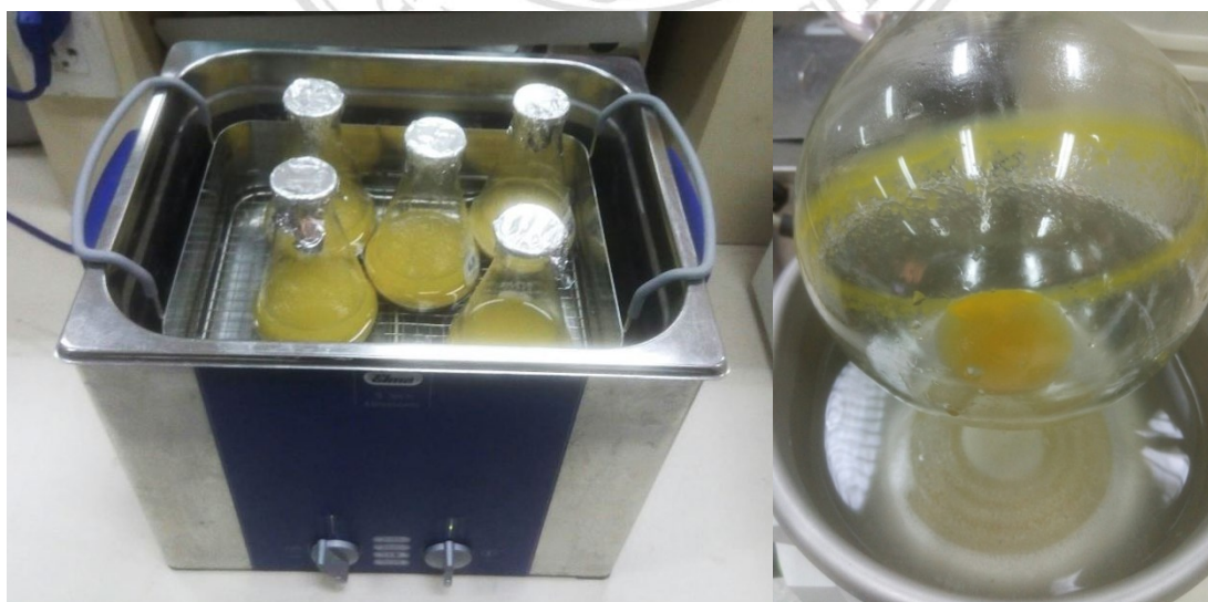
Figure A-2 Soy germ extracted by high power sonication with ethanol 80% (left) and evaporation of ethanol (right)
