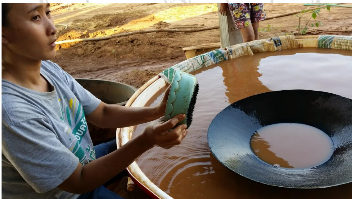
Figure 1 one of the steps of the process of Artisanal mining; the panning, magnetic metal dust removed before the introduction of mercury into the pan.
