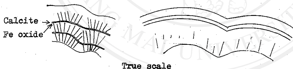
Fig. 2.18 B. The true-scale size of the thin-layered pale purple fluorite described in Fig. 2.18 A. The crystals are radiated perpendicular to the layers. Very thin calcite layers? (cream colour), and Fe oxide layers are interlayered with fluorite.
