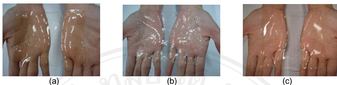
Fig.6. Hydrogel sheets synthesized from AMPS- \text{Na}^+ 50% w/v with 1.0% mol NMBA crosslinker using different methods of initiation: (a) redox initiation, (b) thermal initiation and (c) photoinitiation.
