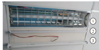
Figure 6. The actual test room with three systems (1) the manual switching system, (2) the fluorescent system, and (3) the LED system
