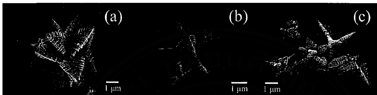
Fig 2. SEM images of the products prepared using (a) 1 : 4, (b) 1 : 1, and (c) 4 : 1 mole ratios of \text{Pb}(\text{NO}_3)_2 to \text{CH}_5\text{N}_3\text{S} , respectively.
