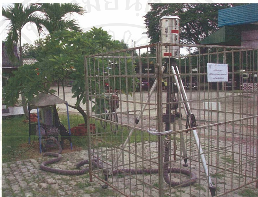
Figure 10 A ChemVol ® Model 4200 high volume cascade impactor, set up in front of Saraphi Hospital, Chiang Mai, to collect particulate matter for four months.
