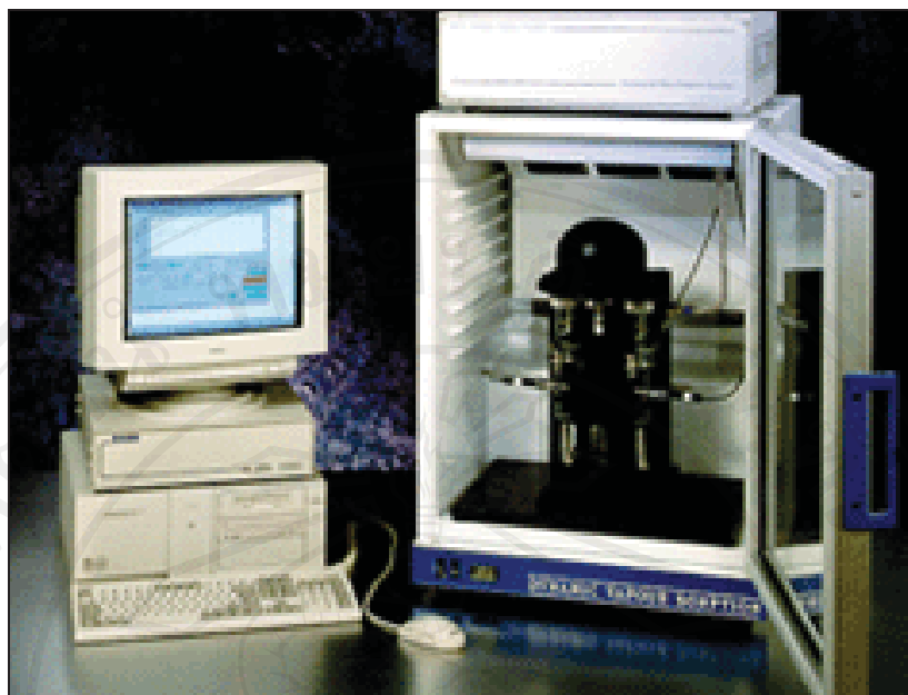
Figure 6.7 : Photograph showing the DVS instrument used in this work.
