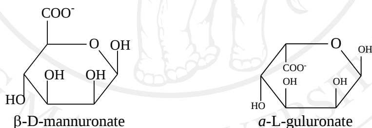
Figure 2.6 The structure of alginate monomers : \beta -D-mannuronate (M) and \alpha -L-guluronate (G)
