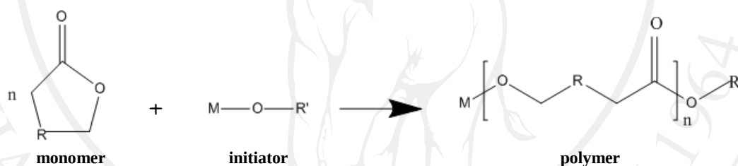
Figure 1.2 : ROP of a cyclic ester monomer using a metal alkoxide (M-OR') as the initiator [4].
